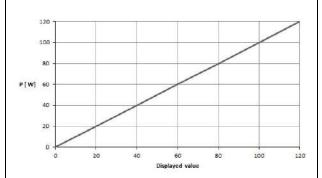
Diagram of power output P [W] as a function of the setting "Monopolar Coagulation Argon flexible" Rated load resistance =  $500 \Omega$
