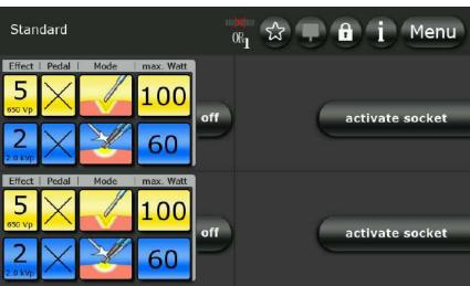
2. On the ARC 400 the connection to OR1 is enabled. There is a correct connection to the OR system. The device can be adjusted from the OR system. The white bar sweeps cyclically from left to right.
