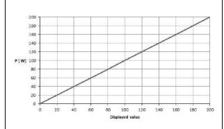
Diagram of power output P [W] as a function of the setting "Bipolar Cutting Standard"
