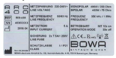
Figure 3-1: Nameplate ARC 400 for 220 - 240 V~
