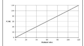
Diagram of power output P [W] as a function of the setting "Bipolar Coagulation Standard forceps AUTOSTART"
