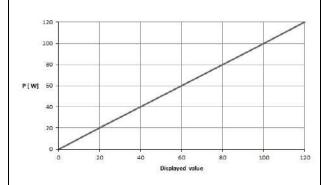
Diagram of power output P [W] as a function of the setting " Bipolar Coagulation bipolar scissors"
