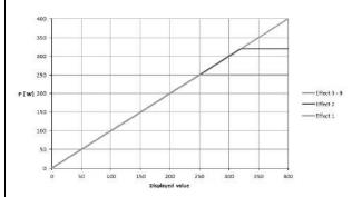
Diagram of power output P [W] as a function of the setting "Monopolar Cutting Standard"
