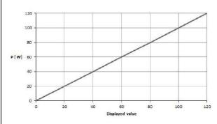
Diagram of power output P [W] as a function of the setting "Monopolar Coagulation Laparoscopy" Rated load resistance = 500  $\Omega$
