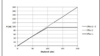
Diagram of power output P [W] as a function of the setting "Monopolar Cutting Laparoscopy"
