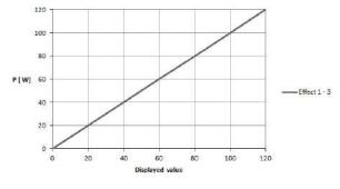
Diagram of power output P [W] as a function of the setting "Monopolar Coagulation Forced mixed" Rated load resistance = 500  $\Omega$
