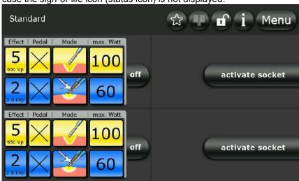
3. On the ARC 400 the connection to TEGRIS is not enabled. In this case the sign-of-life icon (status icon) is not displayed.
