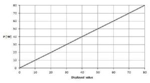
Diagram of power output P [W] as a function of the setting "Monopolar Coagulation Argon flex. pulse" Rated load resistance = 500 Ω
