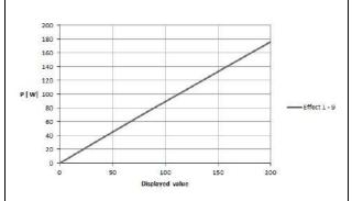
Diagram of power output P [W] as a function of the setting "Monopolar Cutting Dry"
