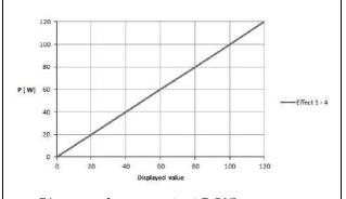
Diagram of power output P [W] as a function of the setting "Monopolar Coagulation Spray"
