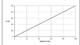
Diagram of power output P [W] as a function of the setting "Monopolar Coagulation Cardiac Thorax" Rated load resistance = 500  $\Omega$
