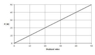
Diagram of power output P [W] as a function of the setting "Monopolar Coagulation GastroCut Coag" Rated load resistance = 500 Ω
