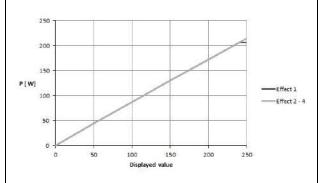
Diagram of power output P [W] as a function of the setting "Monopolar Coagulation Forced cutting" Rated load resistance =  $500 \Omega$
