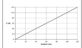
Diagram of power output P [W] as a function of the setting " Bipolar Coagulation Standard forceps " Rated load resistance = 50 Ω
