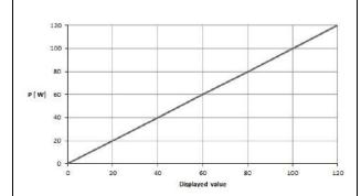
Diagram of power output P [W] as a function of the setting "Monopolar Coagulation Resection"
