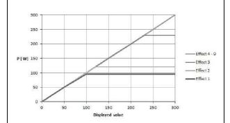
Diagram of power output P [W] as a function of the setting "Monopolar Cutting Argon"
