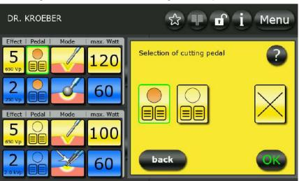
Figure 5-11: Foot switch selection cutting
