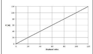
Diagram of power output P [W] as a function of the setting " Bipolar Coagulation Laparoscopy " Rated load resistance = 50 Ω
