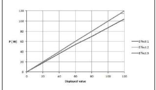
Diagram of power output P [W] as a function of the setting "Monopolar Coagulation SimCoag" Rated load resistance =  $500 \Omega$
