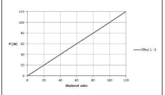
Diagram of power output P [W] as a function of the setting "Monopolar Coagulation Moderate"
