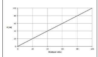
Diagram of power output P [W] as a function of the setting " Bipolar Coagulation forceps forced " Rated load resistance =  $50 \Omega$
