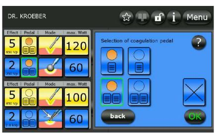
Figure 5-13: Foot switch selection coagulation
