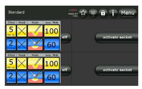
2. On the ARC 400 the connection to TEGRIS is enabled. There is a correct connection to the OR system. The device can be adjusted from the OR system. The white bar sweeps cyclically from left to right.
