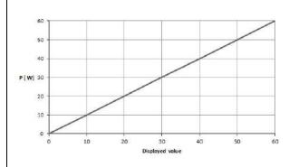
Diagram of power output P [W] as a function of the setting "Monopolar Coagulation Cardiac Mammary" Rated load resistance =  $500 \Omega$
