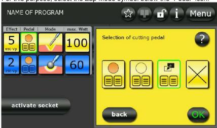
Bild 5-34: Zap Mode foot switch selection for cutting
