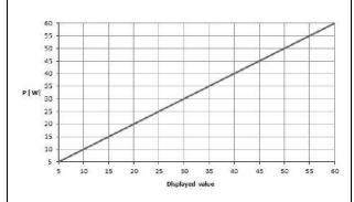
Diagram of power output P [W] as a function of the setting "Bipolar Coagulation SimCoag " Rated load resistance = 50  $\Omega$
