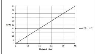
Diagram of power output P [W] as a function of the setting "Monopolar Cutting Micro"
