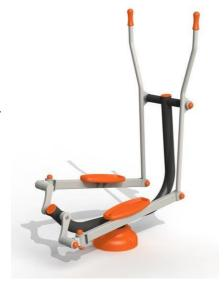
The poles are made of 33 mm diameter pipe with a thickness of 2.8 mm and will be rubber-coated to prevent the limbs from slipping. All moving parts, heads, screws, nuts need to be covered with plastic protective caps. Metal elements need to be sandblasted and electrostatically painted in two layers with a thickness of 100 microns to make them resistant to the external environment.
