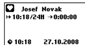
During the recording the display goes out. After short pressing of any button the display lights up for 15 seconds.
