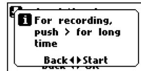
If everything is OK, start recording by long pressing of the enter button
