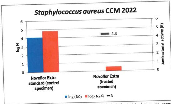
Note: log (N0) ... the logarithm of the mean number of viable bacteria/cm² from the control specimens immediately after inoculation; log (N24) ... the logarithm of the mean number of viable bacteria/cm² from the control and test specimens after incubation for 24 hours; R ... antibacterial activity
