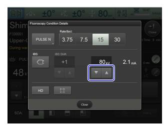
Fluoroscopy tube voltage falls within a range of 50 to 120 kV.
