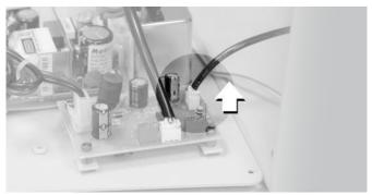
3. Disconnect the LED connection cables from the power supply printed circuit board.
