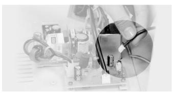
4. Loosen LED board locating ring, take away LED board locating ring.
