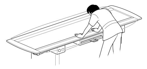
2 Release the foot switch when the tabletop comes to the desired position.
