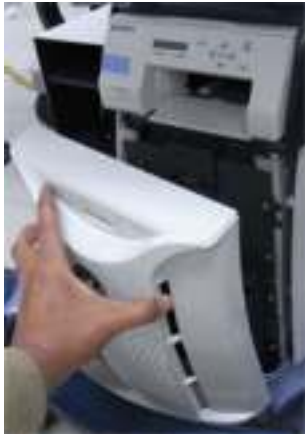
Figure 12-9 • Remove the front cover
