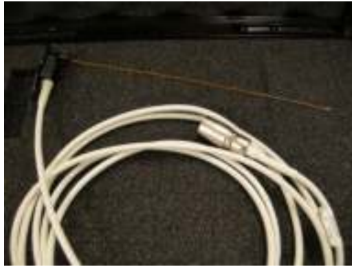
Figure 13-152 • Needle Tip Sensor and Cable Close-up
