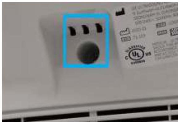
Figure 13-337 • LED location of the battery
