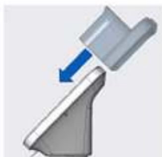
Figure 13-158 • Install Probe Holder on Charger
