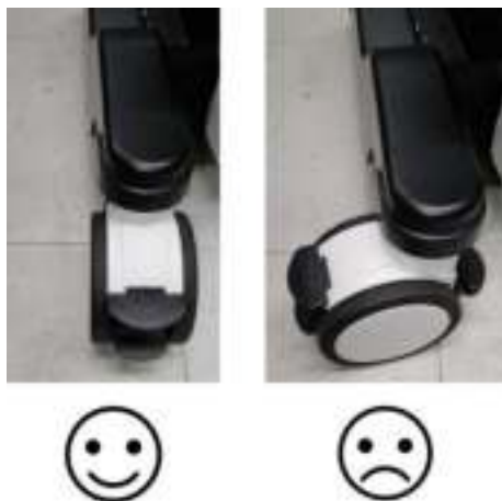
Figure 3-56 • Caster position for Swivel lock
