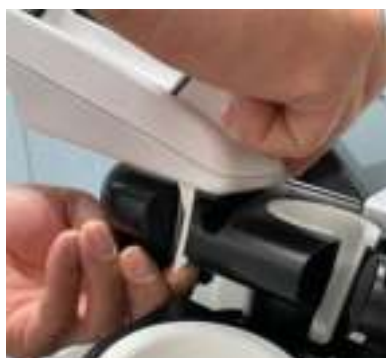
Figure 3-5 • Pull the claw to remove
