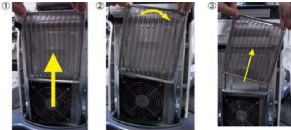
Figure 12-10 • Remove the air filter
