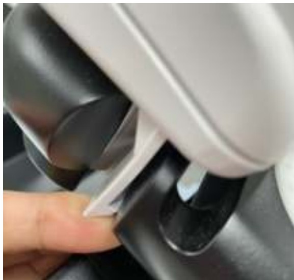
Figure 12-13 • Pull the claw to remove
