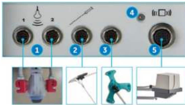
Figure 13-151 • Volume Navigation Connections
