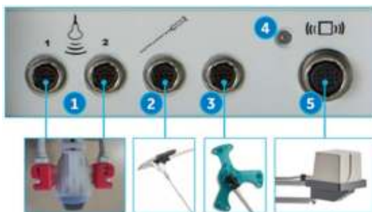
Figure 13-133 • Volume Navigation Connections
