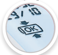
When "OK" symbol appears on the display the cuff is correctly positioned
