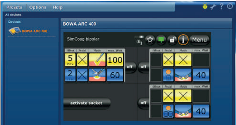
Professionals working together: Set the power, type of current and the activation type through the KARL STORZ OR1™
