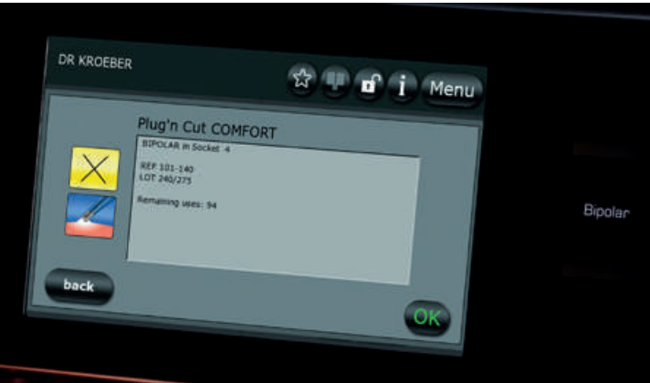
Plug'n Cut COMFORT: The COMFORT SYSTEM automatically recognises the COMFORT instrument, indicates how many times it may still be used and selects the correct parameters for the procedure
