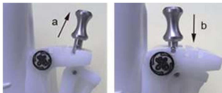
Figure 11-10. Pull up and push down the pin
