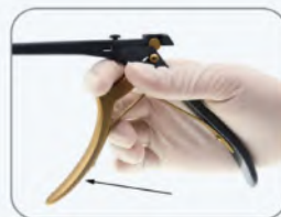
③. Loosen the handle and the detach button at same time to make the positioning pin return within the spring power
