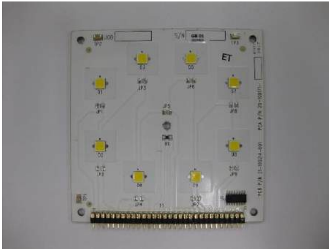
Fig. 1 DURIS S8 load board example.
