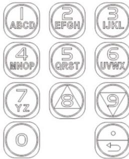
As per above diagram, number key 1 for ABCD, number key 2 for EFGH, number key 3 for IJKL, number key 4 for MNOP, number key 5 for QRST, number key 6 for UVWX, number key 7 for YZ. Press number key “0” to enter numbers 0~9. Press CLEAR key if input wrongly.
