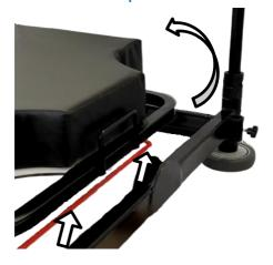
To raise the backrest firstly push gas spring lever upward by two hands and pull up at the same time until it reached desired angle.
