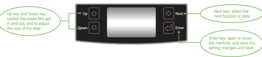
Through the function keys to implement three basic functions: "Shoe Covering" , "Warm Wind" and "Data Adjustment" , these functions can be looping shown by pressing key. See the following figures
