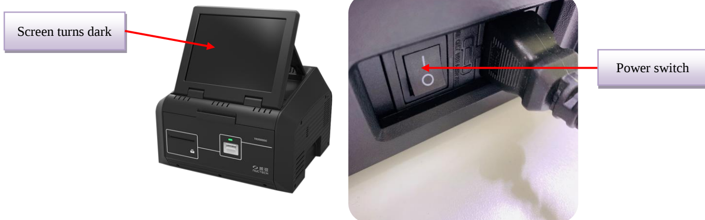
Figure 4.25 Shut down the system
