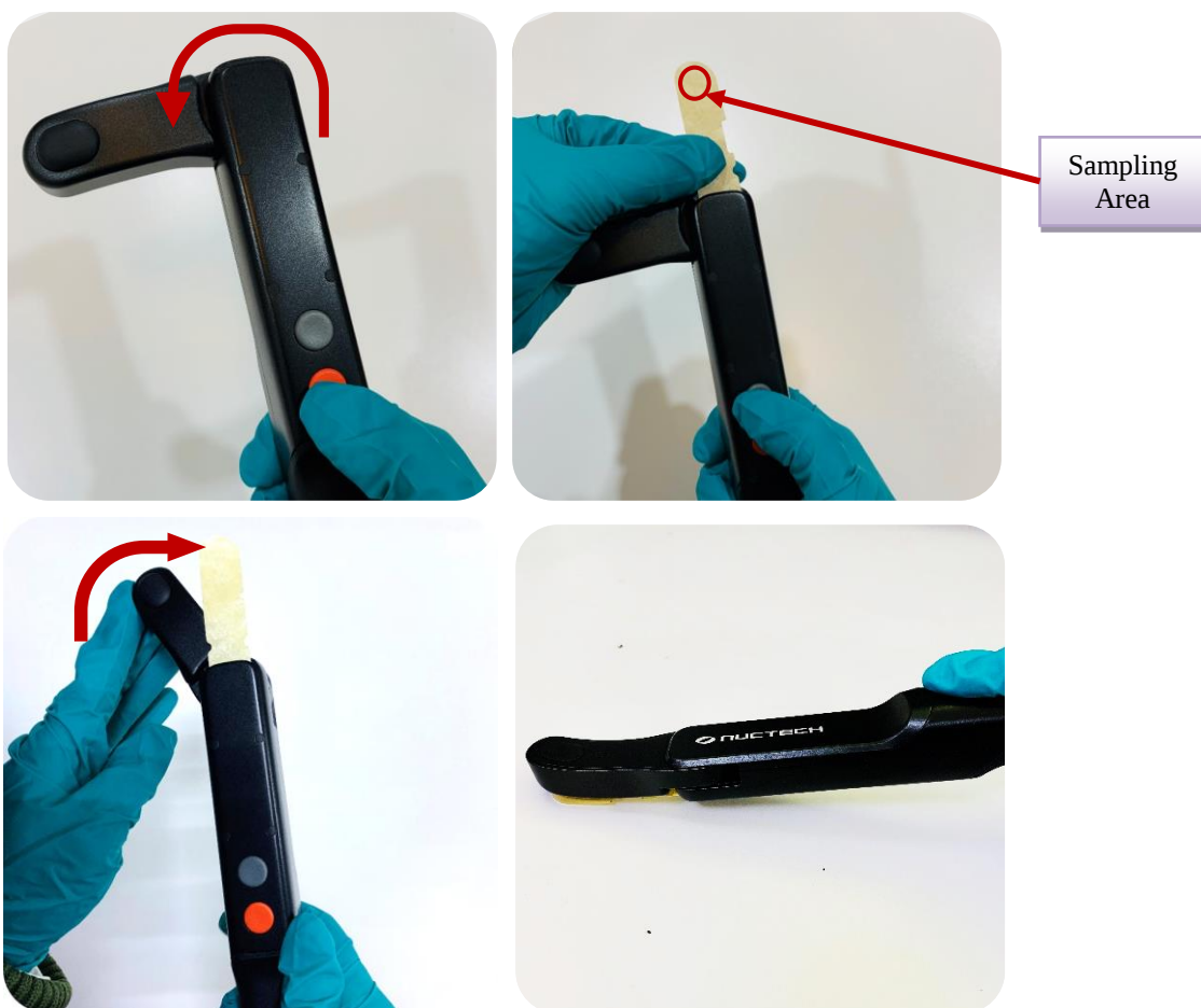
Figure 4.15 Particle sampling with Thumbprint Wand™
