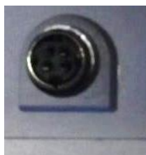
Figure: power supply input (power DIN 4-pin connector)
