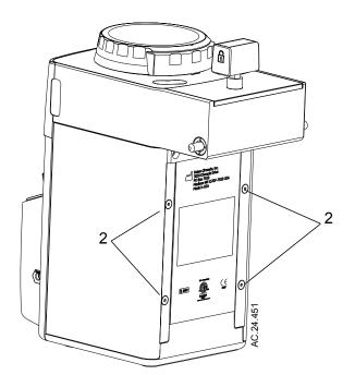
5. Use a screwdriver to pry the Side Plates (3) loose and remove the them (3).
