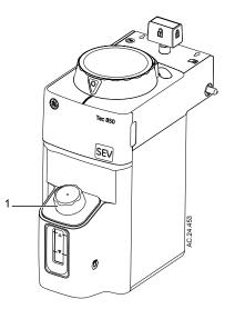
3. Insert a screwdriver between the Snap-On Cover and the filling port to pry off the Snap-On Cover (2).
