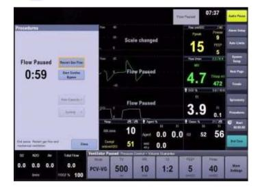
"Flow Paused" indication and countdown time clearly displayed on screen. Press "restart" or tap screen to resume.
