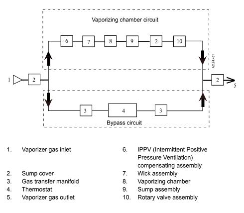
Figure 2-1 • Circuit overview diagram
