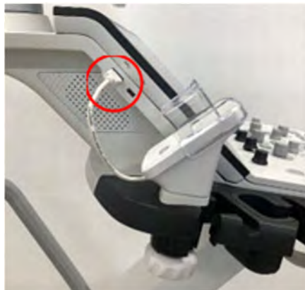
Figure 13-186. LOGIQ Totus USB Ports with Vscan Air CL Probe charger Installed
