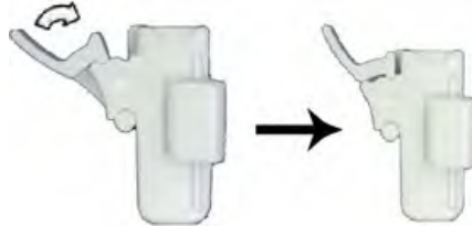
Figure 11-28. Locking the Needle Clip
