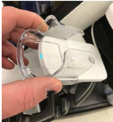
Figure 13-200. Remove Vscan Air Probe Holder
