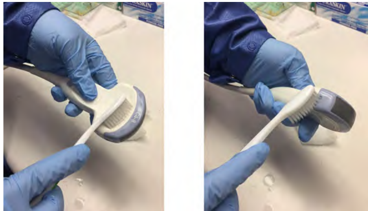
Figure 11-6. Cleaning the probe using a brush
