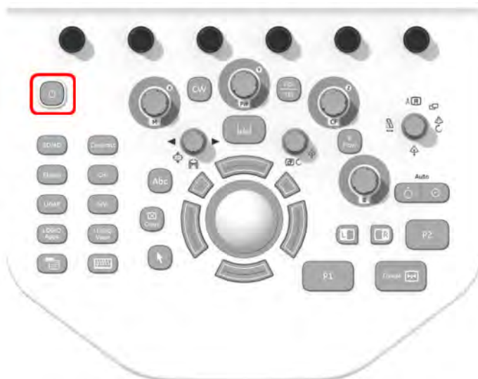
Figure 3-9. Power On/Off Switch Location
