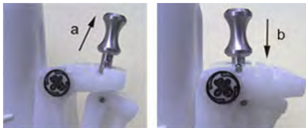
Figure 11-33. Pull up and push down the pin
