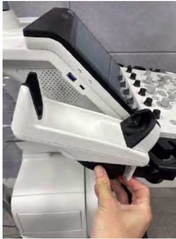
Figure 3-6. Pull the hook to disassemble the probe holder
