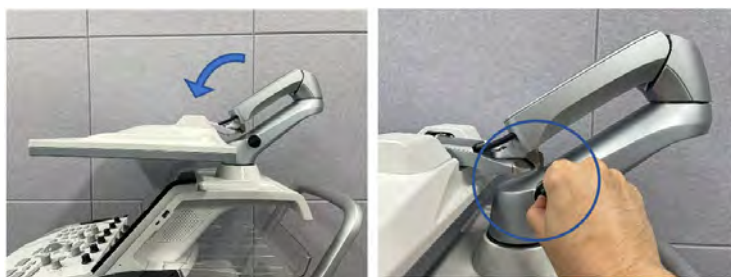
Figure 3-40. Flip down the monitor and lock the monitor arm
