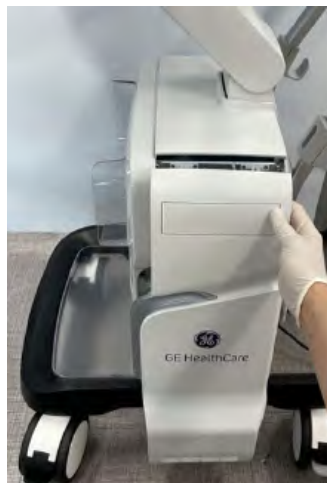
Figure 12-11. Remove the side cover left or right
