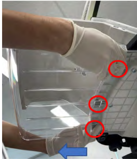
Figure 12-14. Disassemble the Control panel rear tray
