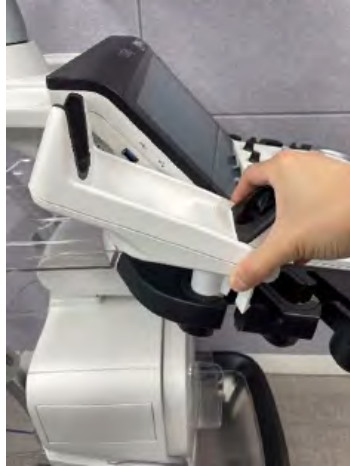
Figure 3-4. Install TVTR Probe holder
