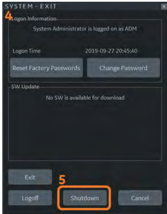
Figure 13-274. Shutdown to Begin Installation
