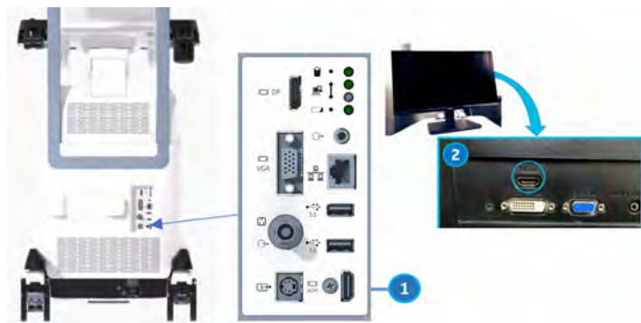
Figure 3-7. Connect HDMI Cable to back of LOGIQ Totus and External Monitor
