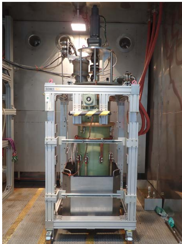
Picture 2: Test setup in a climatic chamber for the operation tests at -25 °C and 115 °C and the operation test at maximum allowable static pressure.
