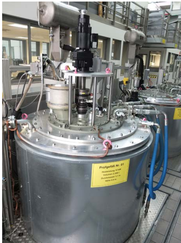
Picture 1: Test setup for the mechanical endurance test (heatable test vessel).
