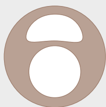
Dual-lumen catheter shaft
