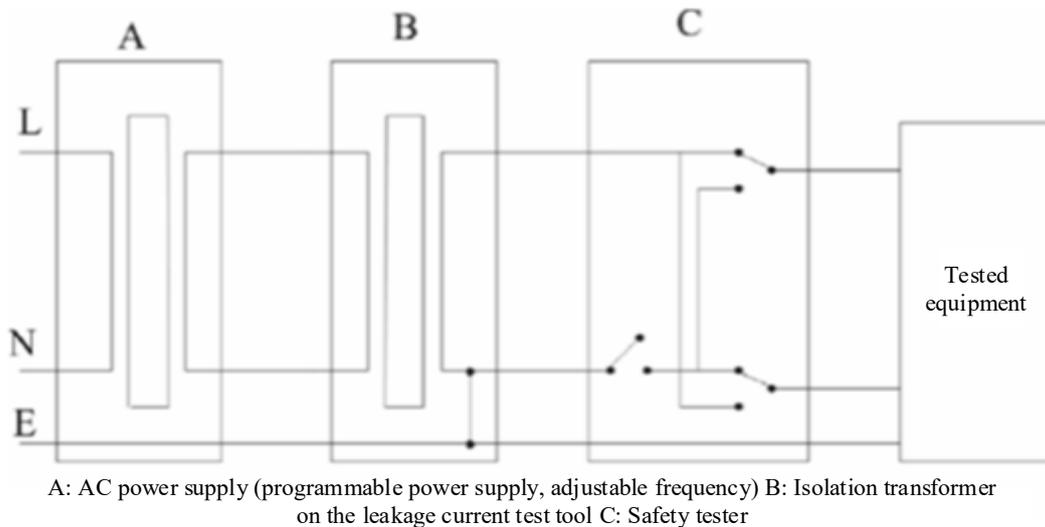
**Figure 7-3 Device Connection Diagram**
