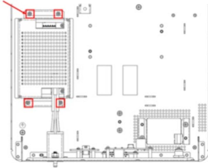
**Figure 9-8 Disassembling the AC-DC Module**
