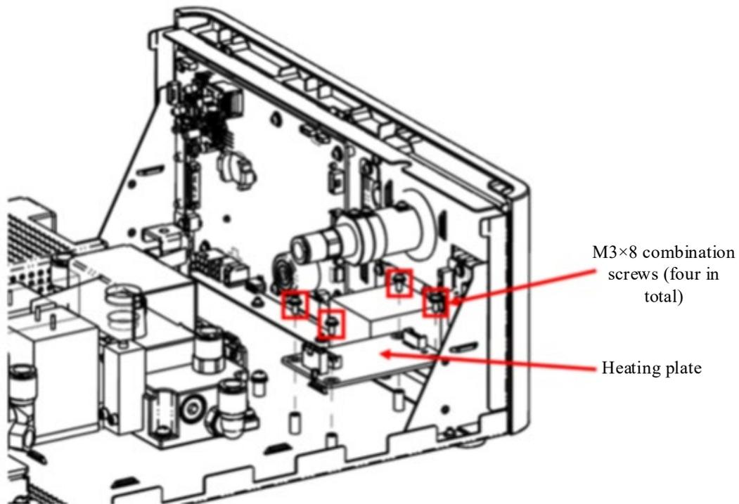
Figure 9-16 Disassembling the Heating Plate
