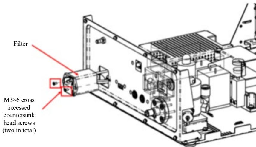
Figure 9-4 Disassembling the Filter Assembly
