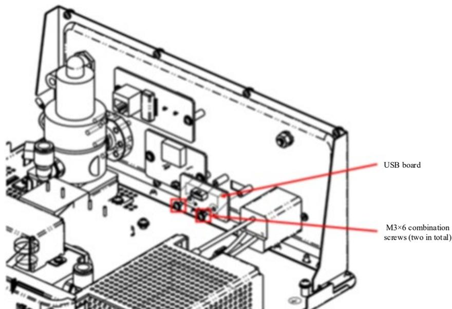
Figure 9-17 Disassembling the USB Board
