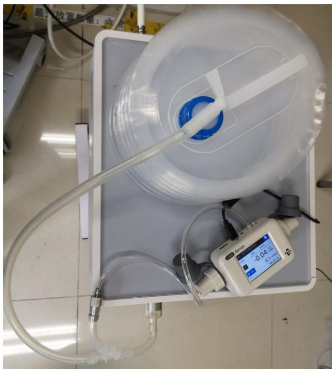
**Figure 7-1 Pressure Test Connection Diagram**
