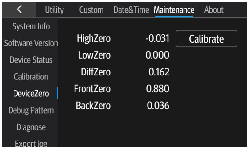
**Figure 6-5 Calibration for High-Pressure Sensor of Insufflator V2.0**
