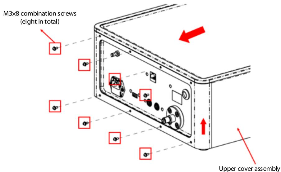
**Figure 9-1 Disassembling the Upper Cover Assembly**
