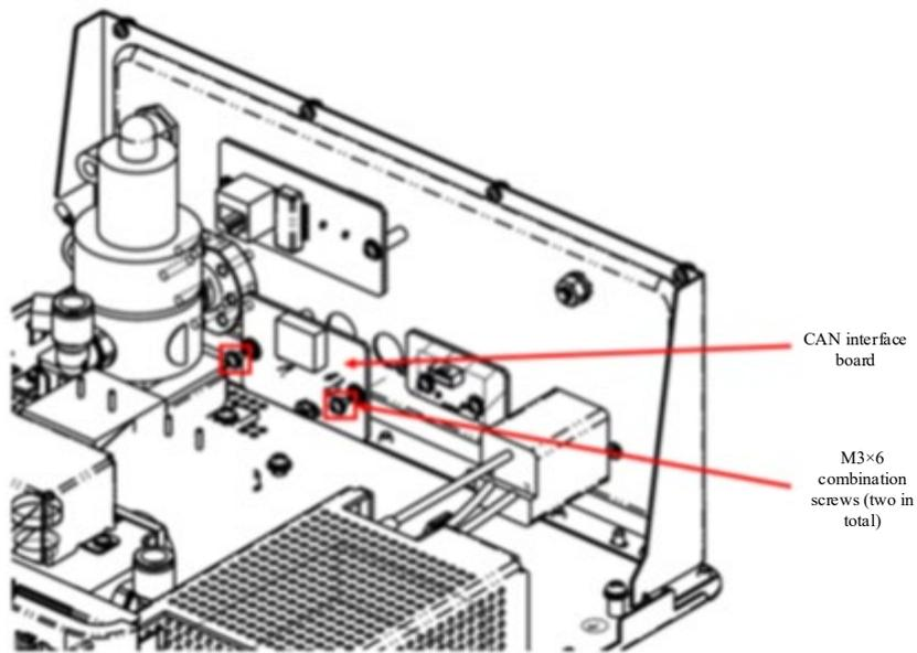
**Figure 9-18 Disassembling the CAN Board**
