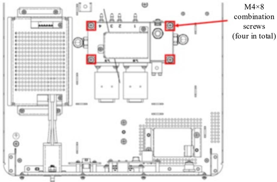
Figure 9-6 Disassembling the Pressure Relief Valve Assembly
