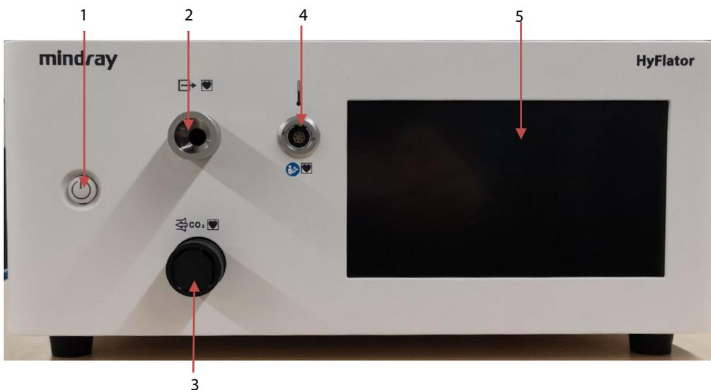
**Figure 2-1 Front Panel of Insufflator**
