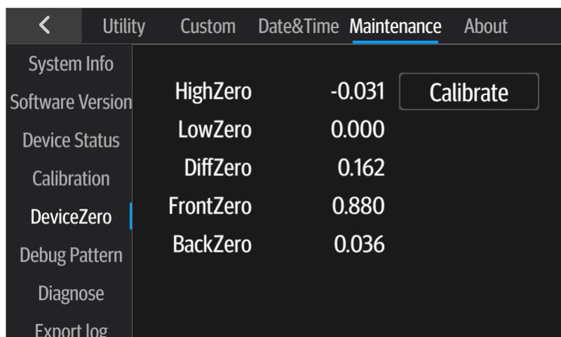
**Figure 5-22 Device Zero Interface**
