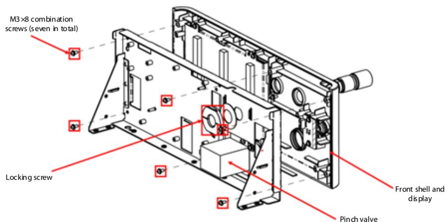
Figure 9-13 Disassembling the Front Shell and Display
