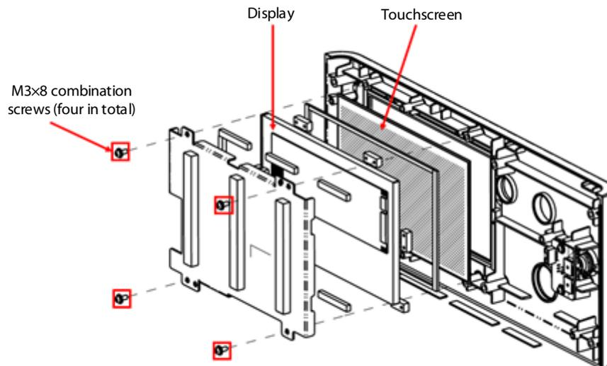
Figure 9-14 Disassembling the Display and Touchscreen
