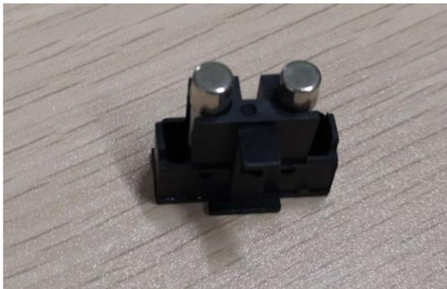
**Figure 9-25 Disassembling the Fuse**
