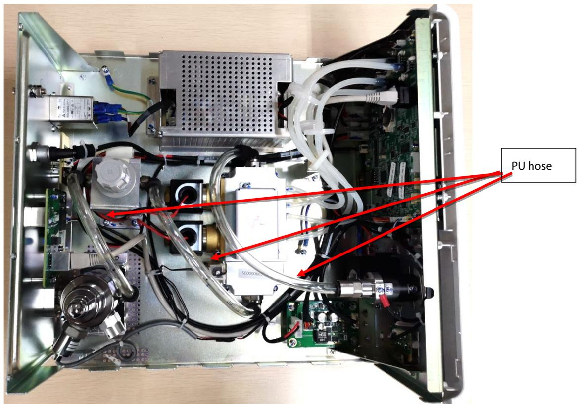
Figure 9-24 Replacing the PU Hose
