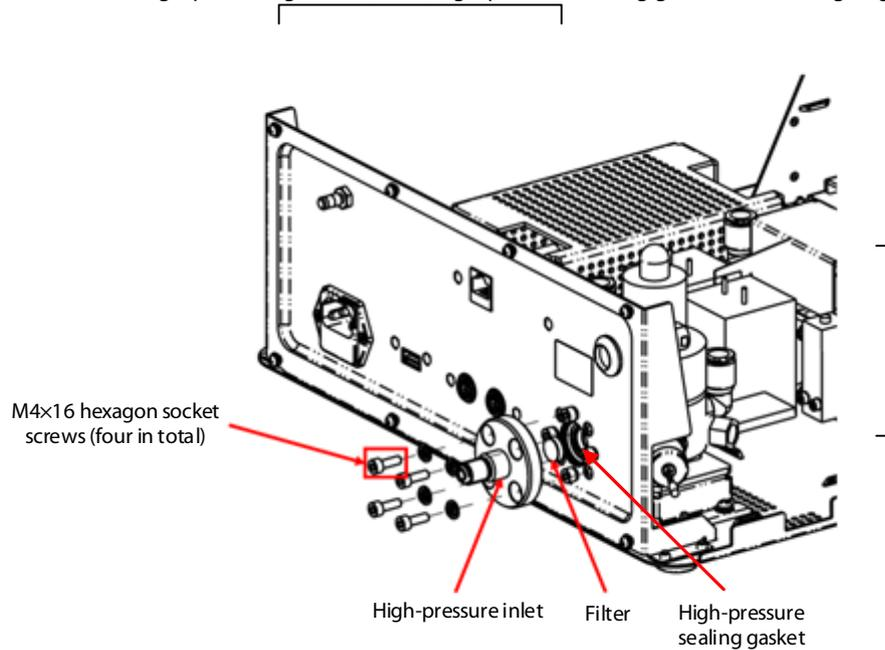
Figure 9-2 Disassembling Gas Inlet and Filter
