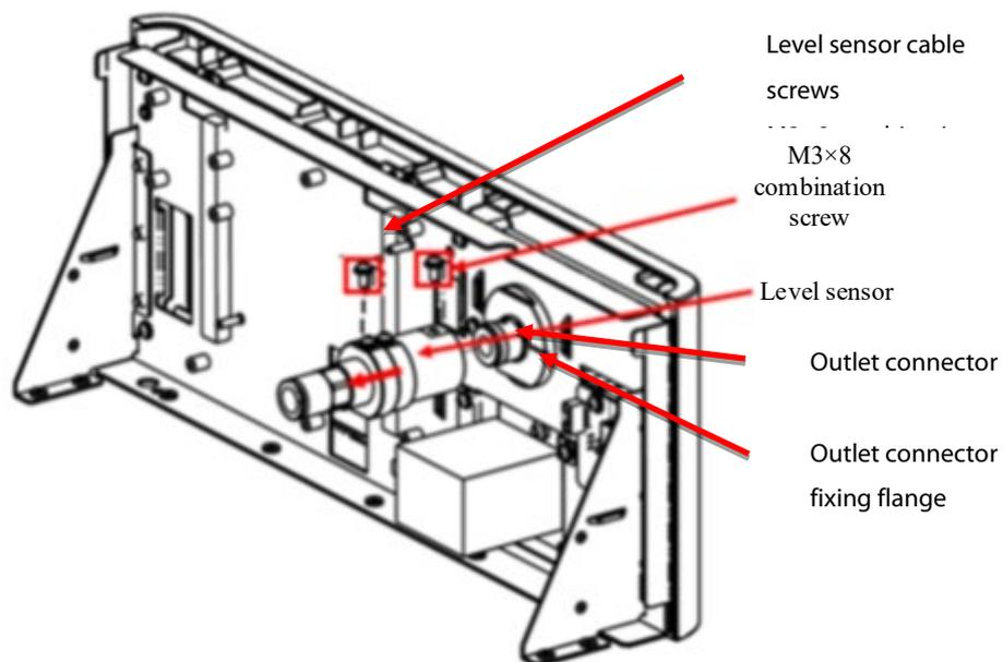
Figure 9-12 Disassembling the Liquid Sensor and Outlet Connector
