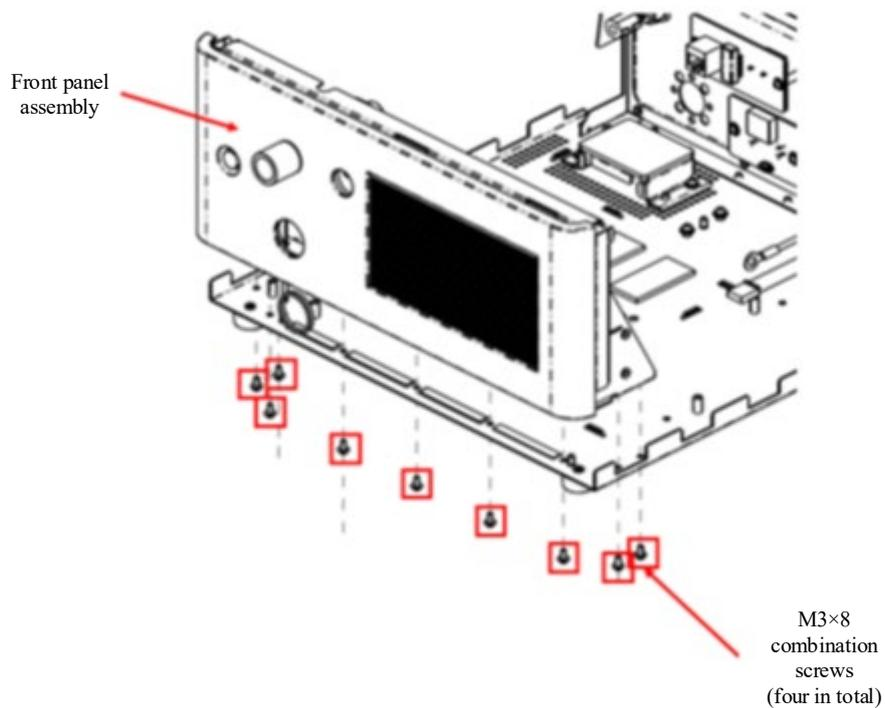
Figure 9-10 Disassembling the Front Panel
