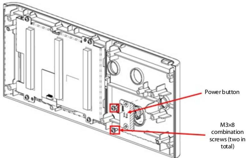
Figure 9-15 Disassembling the Display and Touchscreen
