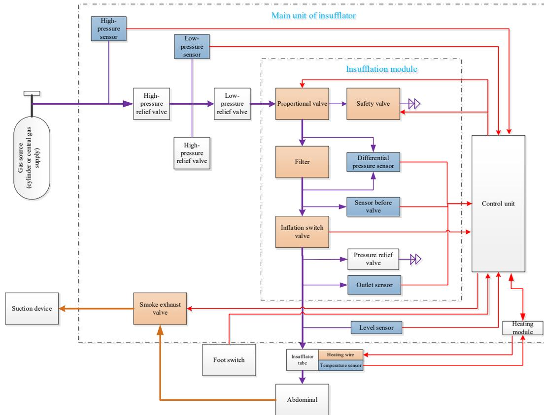
**Figure 2-3 System Block Diagram of Insufflator**
