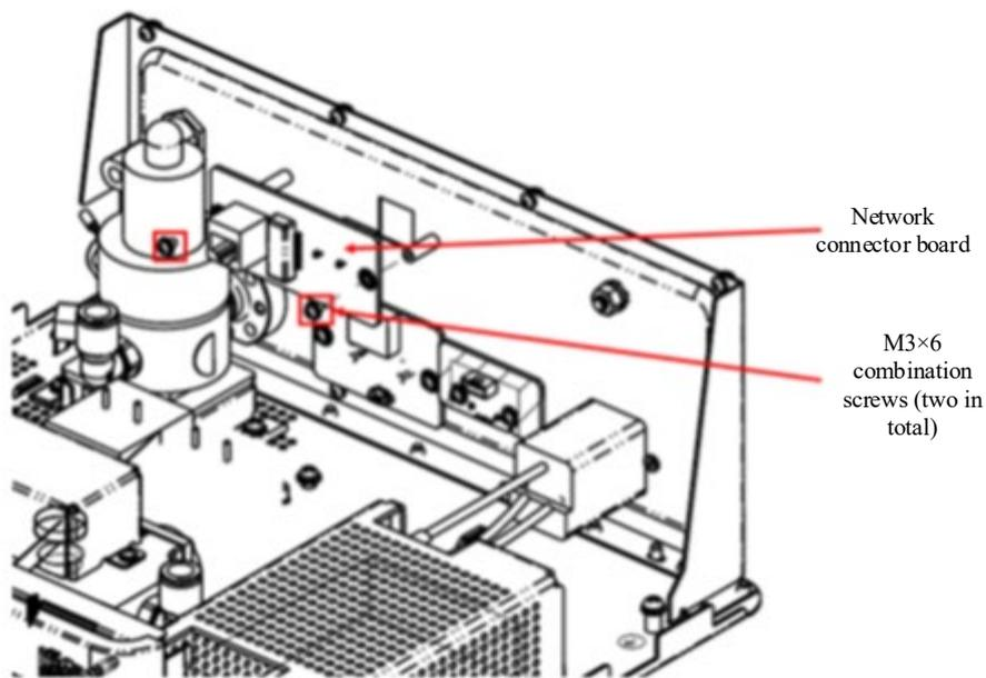
**Figure 9-19 Disassembling the Network Connector Board**
