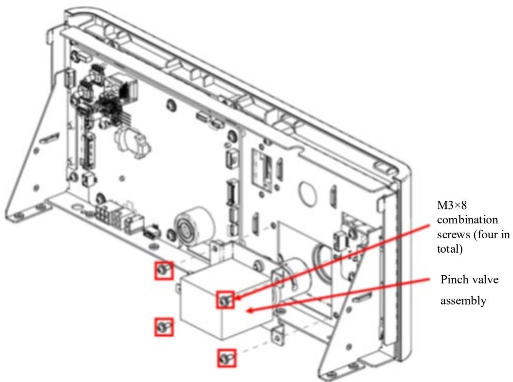
**Figure 9-20 Replacing the Pinch Valve**
