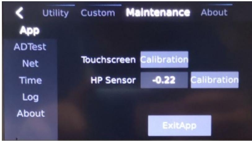
2. Tap the **Calibration** control on the screen. There will be five cross points on the upper left, upper right, lower right, lower left and middle of the screen. Please tap the center of the cross points exactly, as shown in the figure below.
