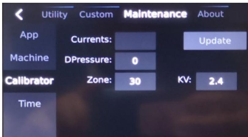
Figure 5-8 Factory-Calibrator Interface
