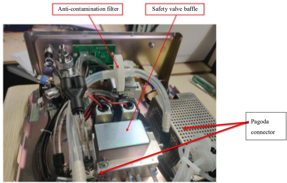
Figure 9-23 Disassembling the Anti-contamination Filter Assembly
