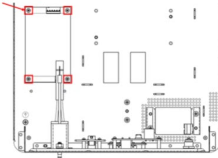
**Figure 9-9 Disassembling the AC-DC Module**
