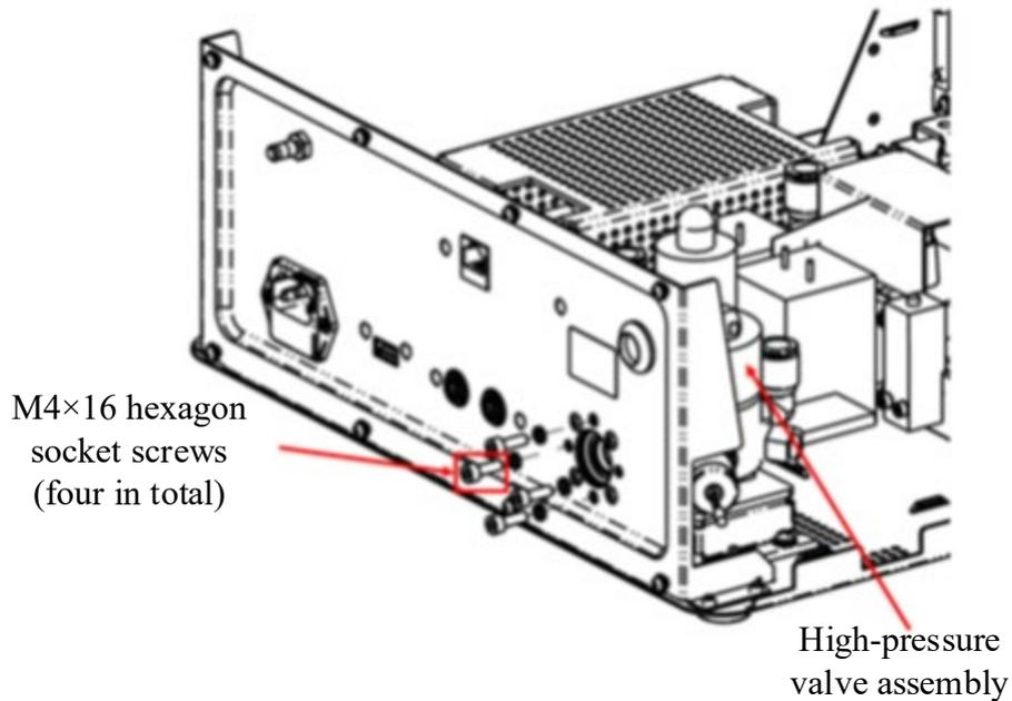
**Figure 9-3 Disassembling the High-pressure Valve Assembly**
