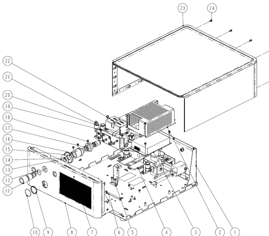
**Figure 2-4 Mechanical Structure Diagram of Insufflator**
