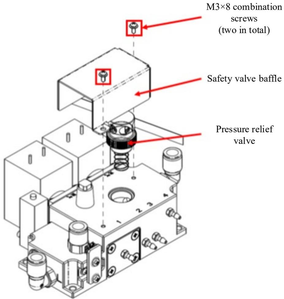
Figure 9-7 Disassembling the Pressure Relief Valve
