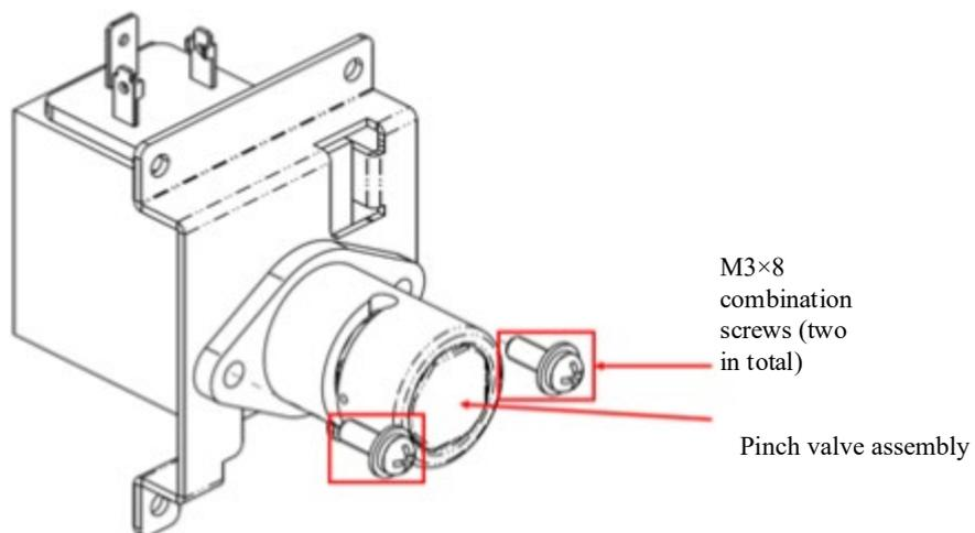
**Figure -21 Disassembling the Pinch Valve**
