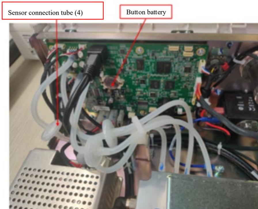
Figure 9-22 Disassembling the Sensor Connection Tubes
