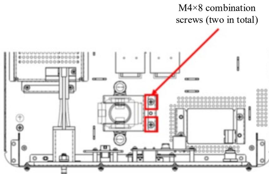
Figure 9-5 Disassembling the Low-pressure Valve Assembly
