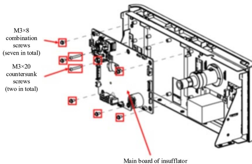
**Figure 9-11 Disassembling the Main Board**
