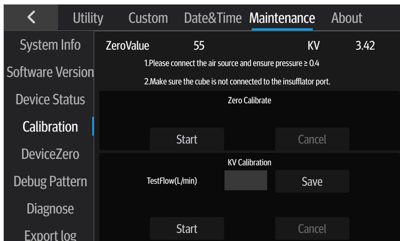
**Figure 6-9 KV Calibration**
