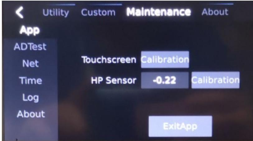
**Figure 6-4 Calibration for High-Pressure Sensor of Insufflator V1.0**
