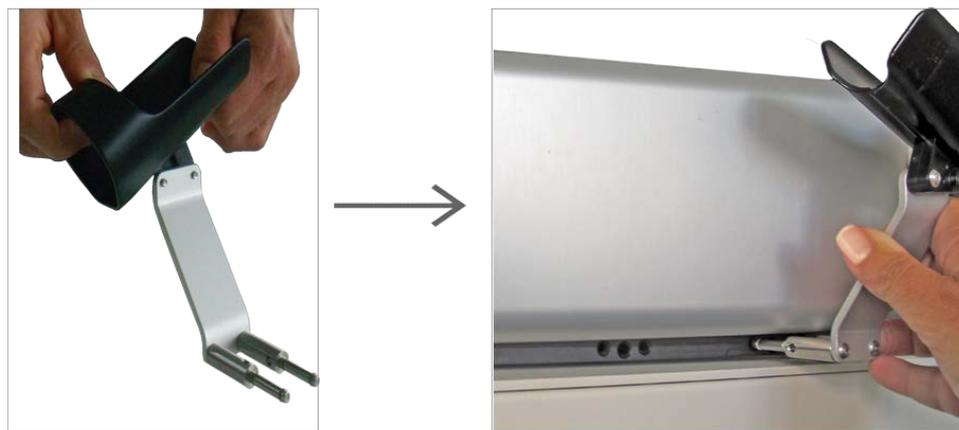
Fig. 3-2 Handpiece holder installation
