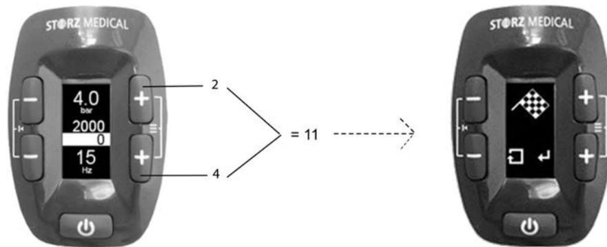
Fig. 9-4 Button combination 11: Switch to the main menu
