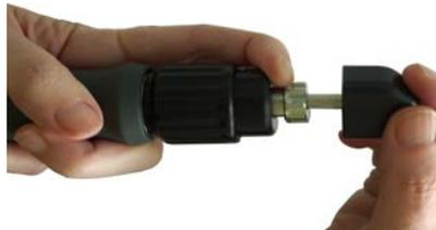
Fig. 9-8 Disassembling the spine or fascia pulse transmitter
