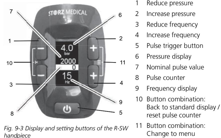
Fig. 9-3 Display and setting buttons of the R-SW handpiece
