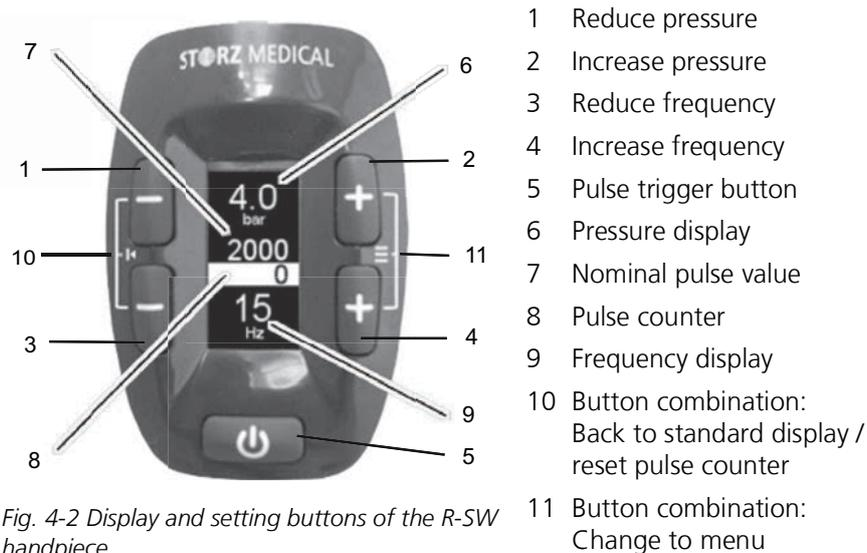
Fig. 4-2 Display and setting buttons of the R-SW handpiece
