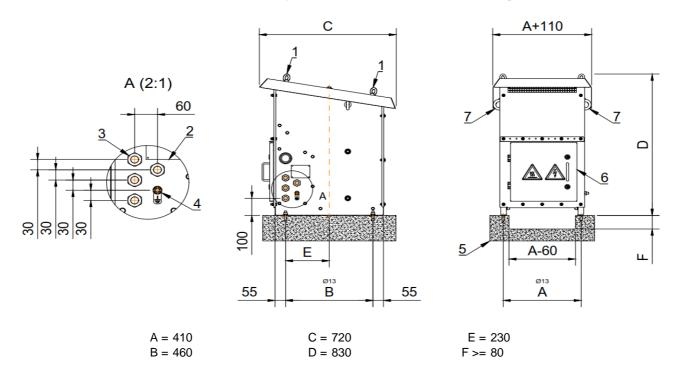
Dimensions LxWxH: 720 x 520 x 830 mm Weight: 74 kg
