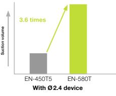
The 3.2 mm working channel provides greater suction performance than conventional models.\*
