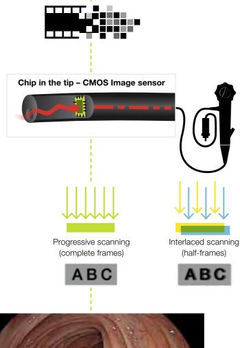
The CMOS chip is positioned directly in the tip of the endoscope and transforms the analogue signal into a digital signal at the site of examination. This ensures brilliant image transmission with reduced noise.
