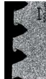
Deformed taper structure after 61 months in vivo
