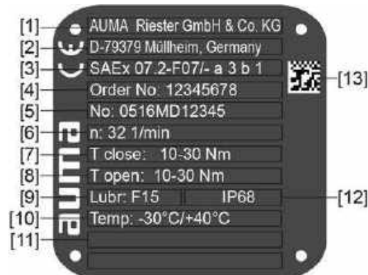
Figure 2: Actuator name plate (example)
