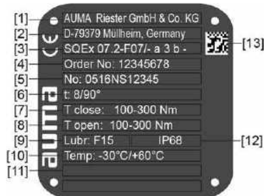
Figure 2: Actuator name plate (example)
