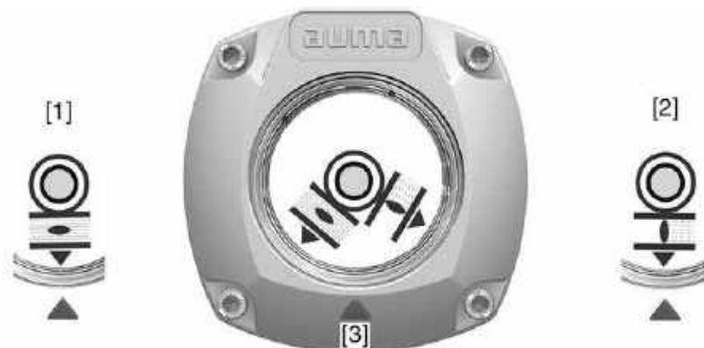
Figure 76: Mechanical position indicator
