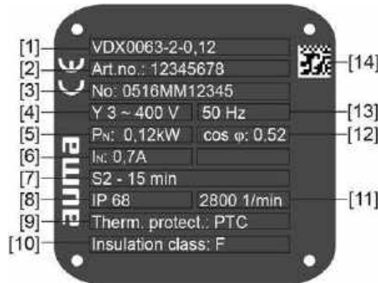
Figure 3: Motor name plate (example)
