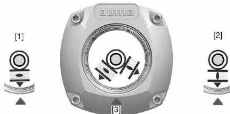
Figure 32: Mechanical position indication via indicator mark on cover
