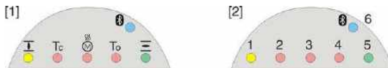
Figure 74: Arrangement and signification of indication lights
