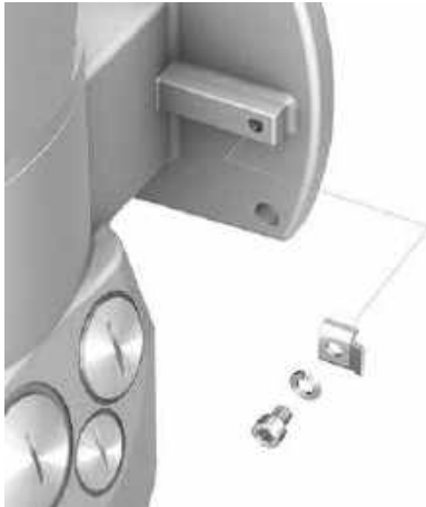
Figure 42: Earth connection for wall bracket
