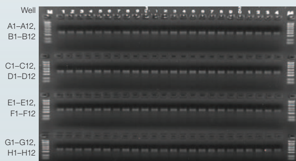
Obtain consistent results with low sample volumes. A 300 bp product was amplified from genomic DNA in 5\ \mu\text{l} reactions. M, markers.
