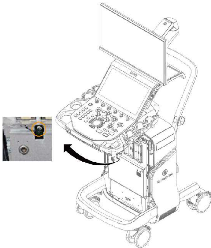
Figure 12-259 Disconnecting Protector Assy's Connector
