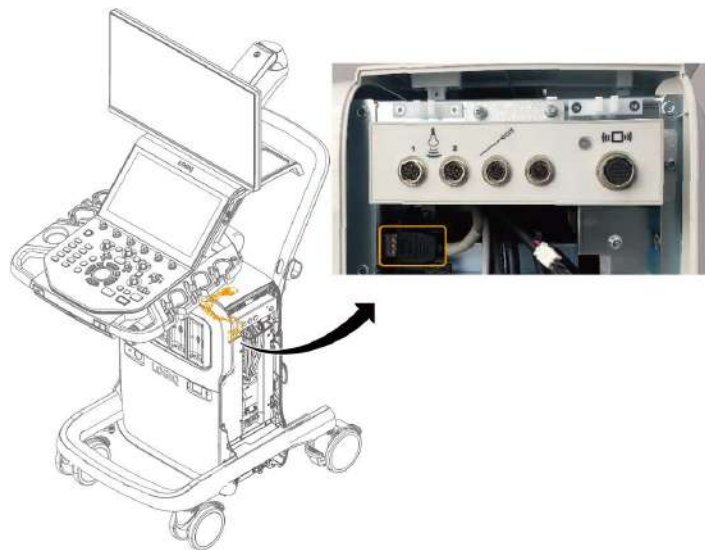
Figure 12-286 Disconnecting UCO TO V NAV SIGNAL CABLE
