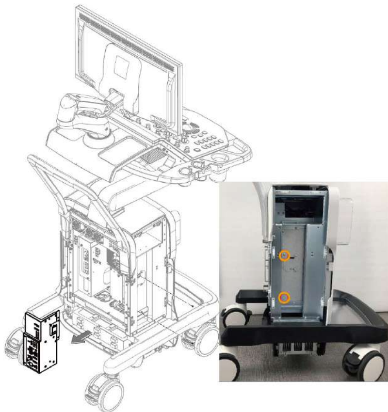
Figure 12-136 Removing UEPP Assy module
