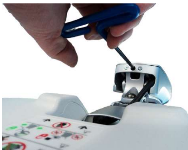
Figure 5-7 Turn the adjustment screw
