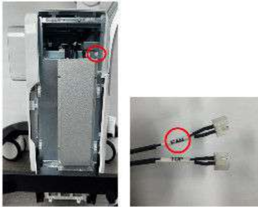
Figure 12-150 Checking Label "FAN"
