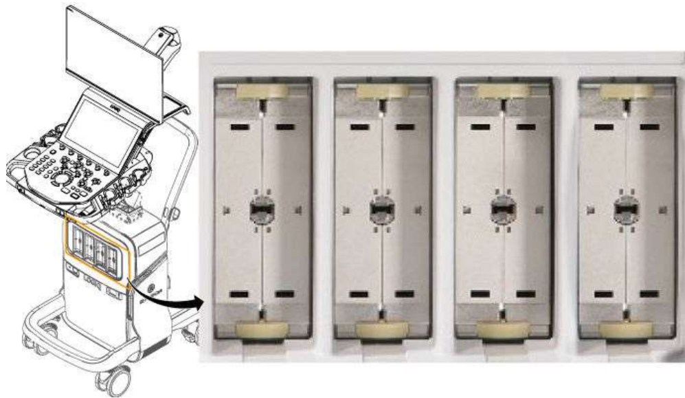
Figure 4-7 Probe Connectors, Four DLP Probe Ports
