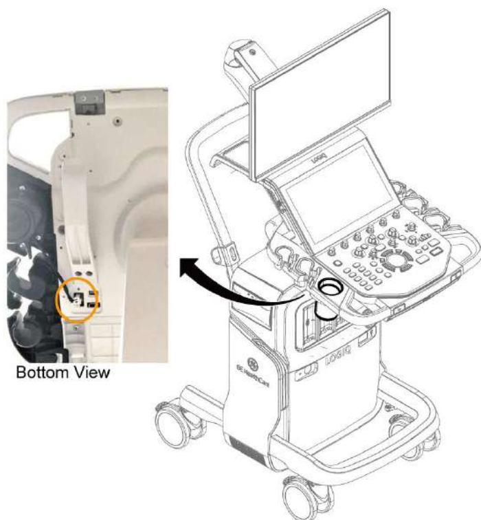
Figure 12-237 Disconnecting cable for T2 Gel Warmer
