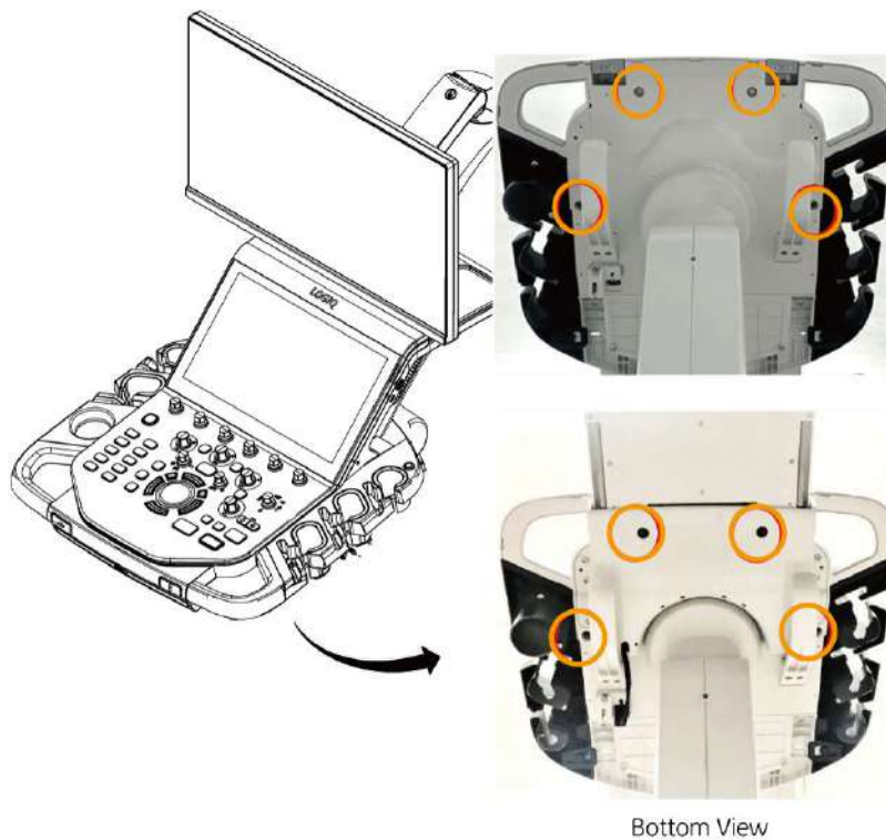
Figure 12-59 Unscrewing bottom screws
