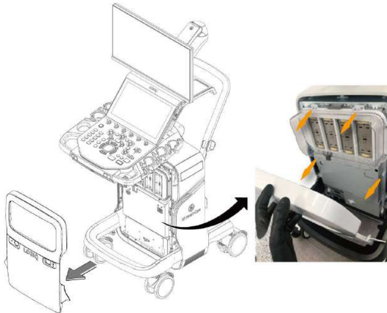
Figure 1-6 Removing Front Cover
