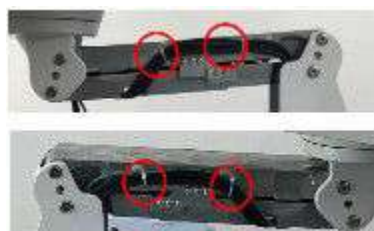
Figure 12-217 Cutting Cable Ties
