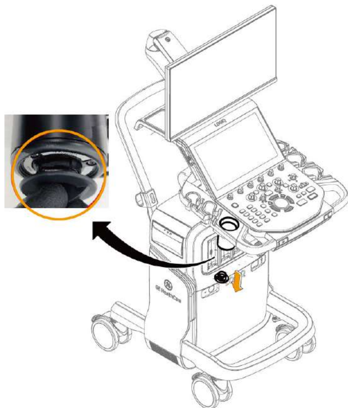
Figure 12-239 Removing Gel Warmer Cap
