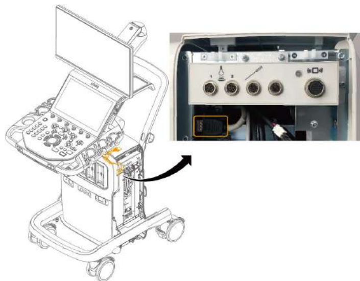
Figure 12-106 Disconnecting UCO TO V NAV SIGNAL CABLE
