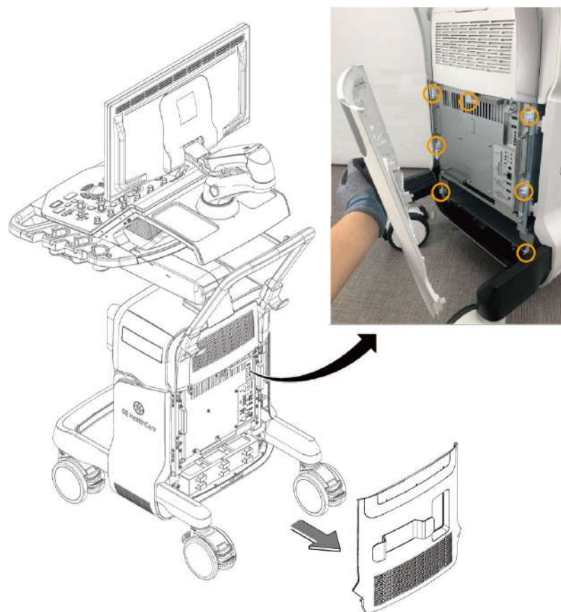
Figure 12-11 Removing Rear Cover Mid Assy
