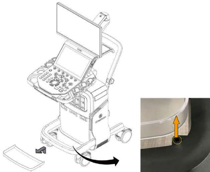
Figure 1-5 Removing Base Tray
