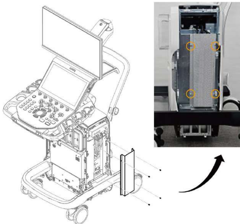
Figure 12-171 Removing Cable Cover Brkt
