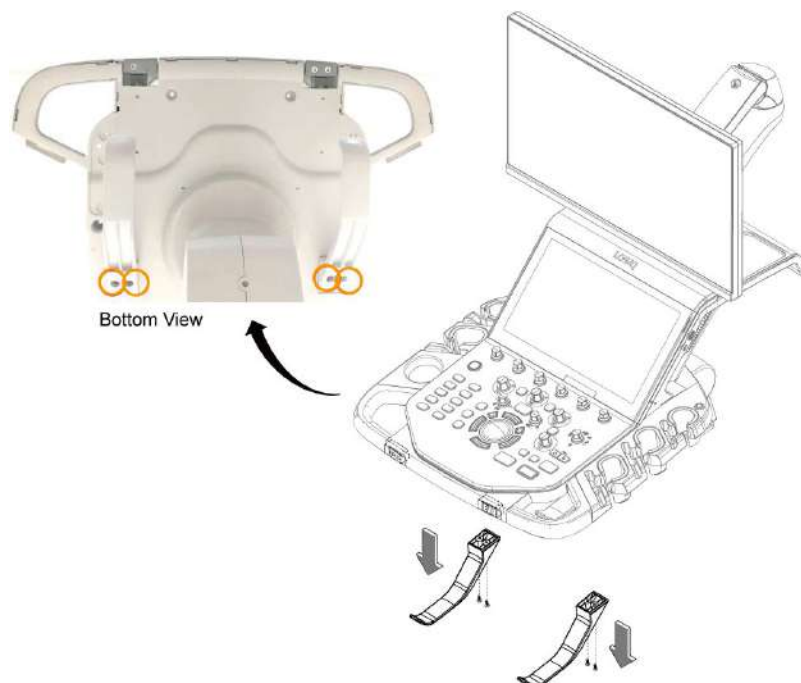
Figure 12-65 Removing OPIO Cable Hook
