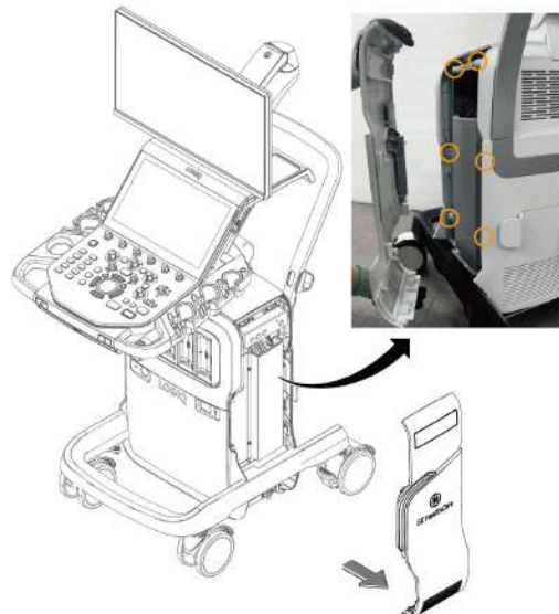
Figure 12-105 Removing T2 SIDE COVER ASSY RIGHT
