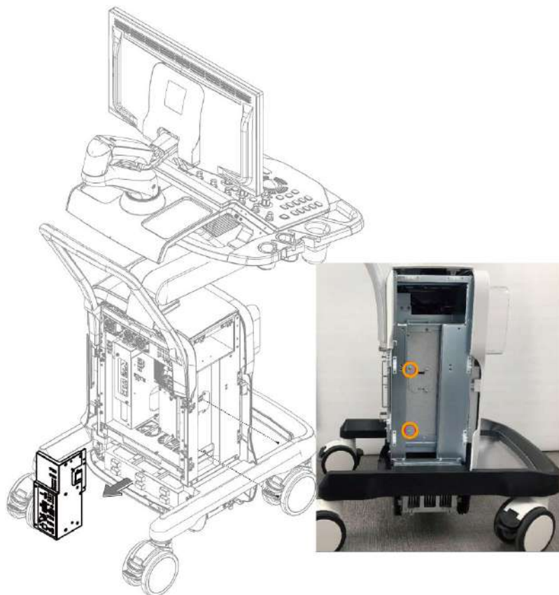
Figure 12-282 Removing UEPP Assy
