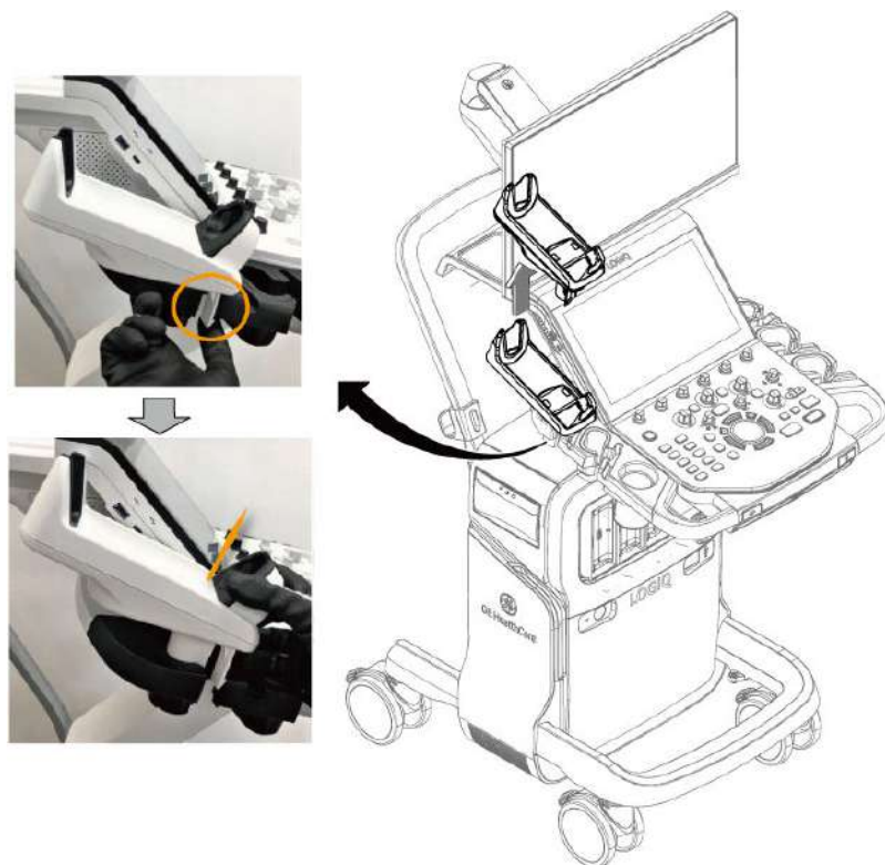
Figure 12-250 Removing TVTR Probe Holder
