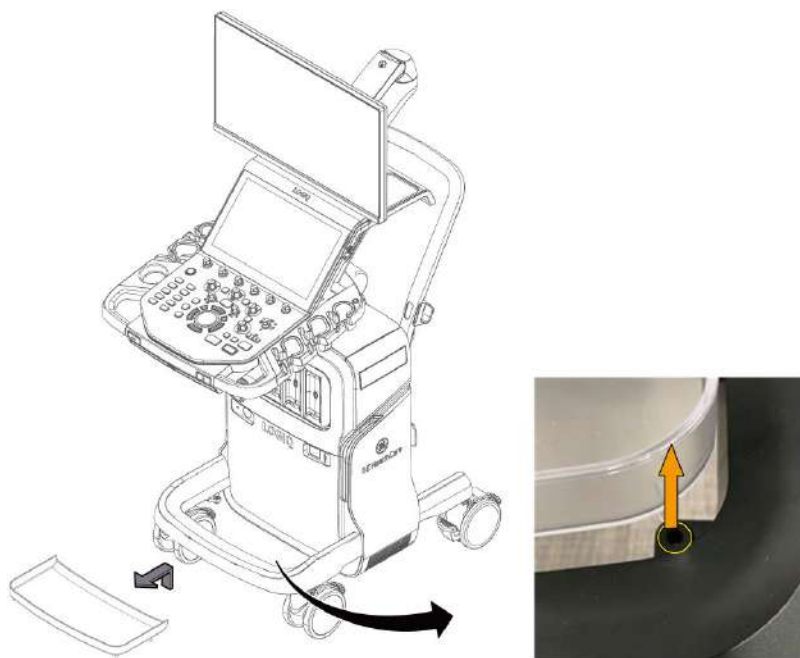
Figure 12-25 Removing Base Tray
