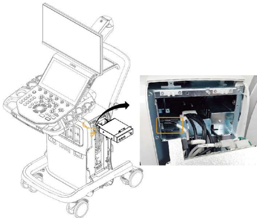
Figure 12-268 Disconnecting Signal Cable
