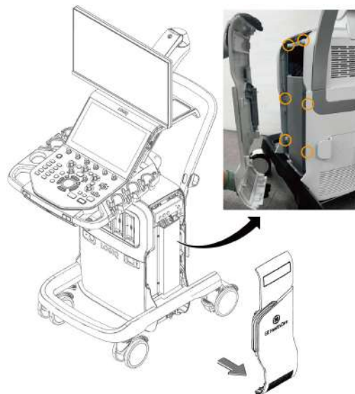
Figure 12-285 Removing T2 SIDE COVER ASSY RIGHT
