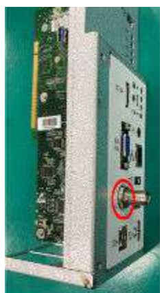
Figure 12-283 Unscrewing Nut from VNC connector
