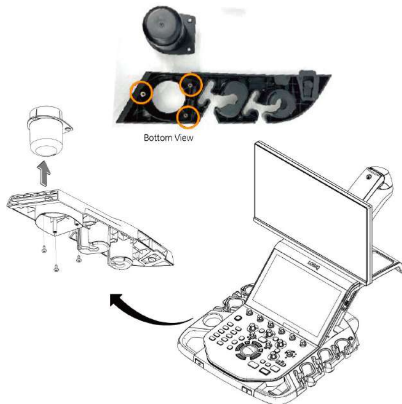
Figure 12-52 Removing Gel Holder
