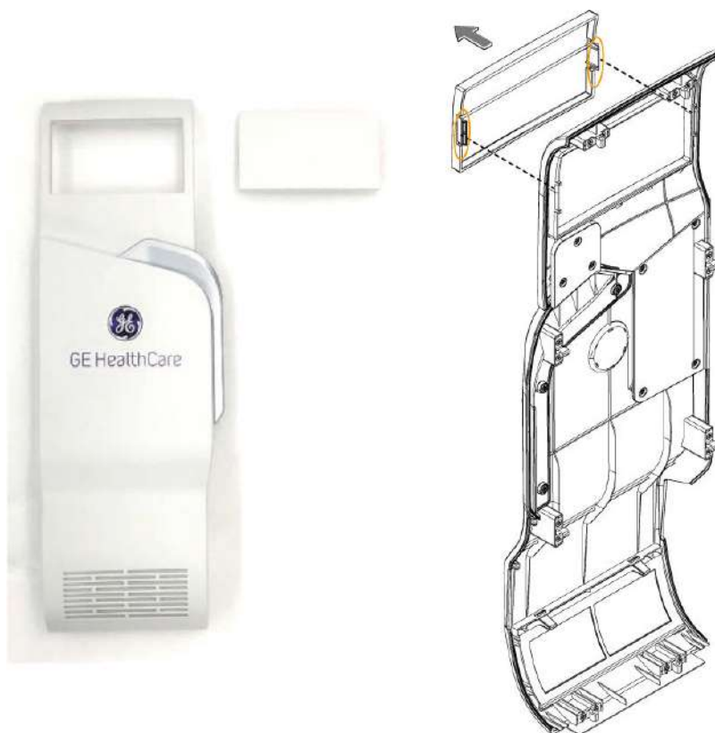
Figure 12-9 Removing BW Dummy Cover
