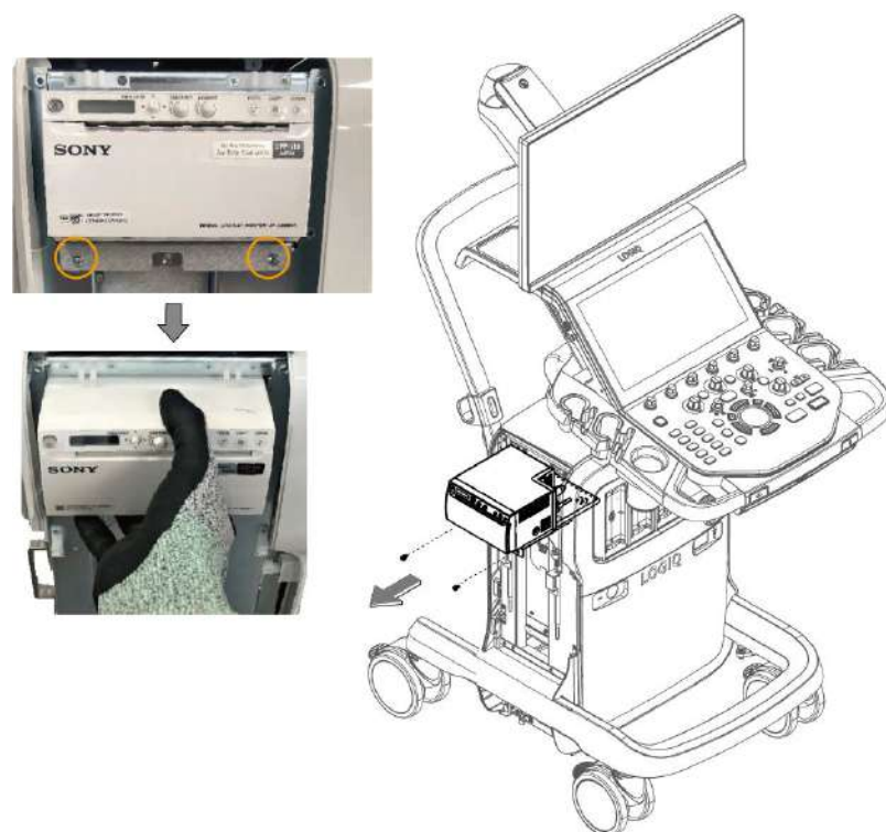
Figure 12-257 Removing BW Printer Assy
