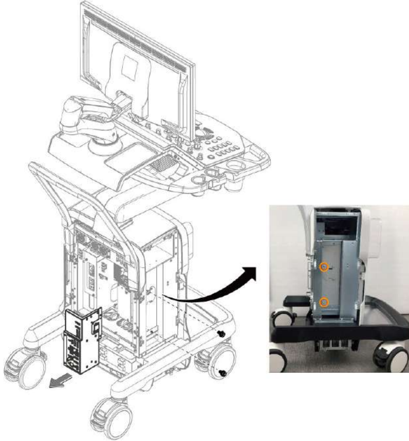
Figure 12-146 Removing UEPP Assy module
