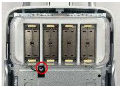
Figure 12-112 Disconnecting Protector Assy's Connector
