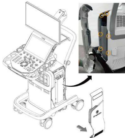
Figure 12-110 Removing T2 SIDE COVER ASSY RIGHT
