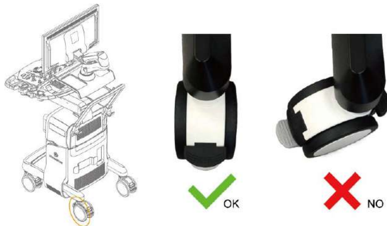
Figure 6-13 Caster position for Swivel lock
