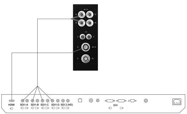
You can connect the Sony monitor to the device via the SDI connection sockets or via the HDMI connection sockets.
