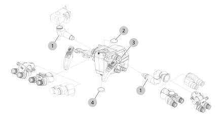
Figure 82: Attaching the documentation/co-observation system
