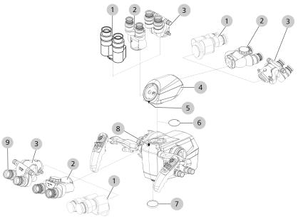
*Figure 81: Attaching the tubes and eyepieces*
