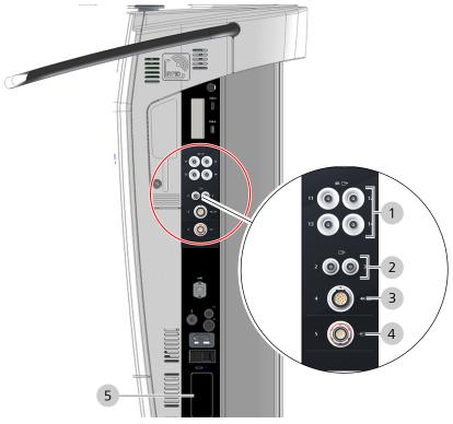
Figure 10: Overview of video connector panel
