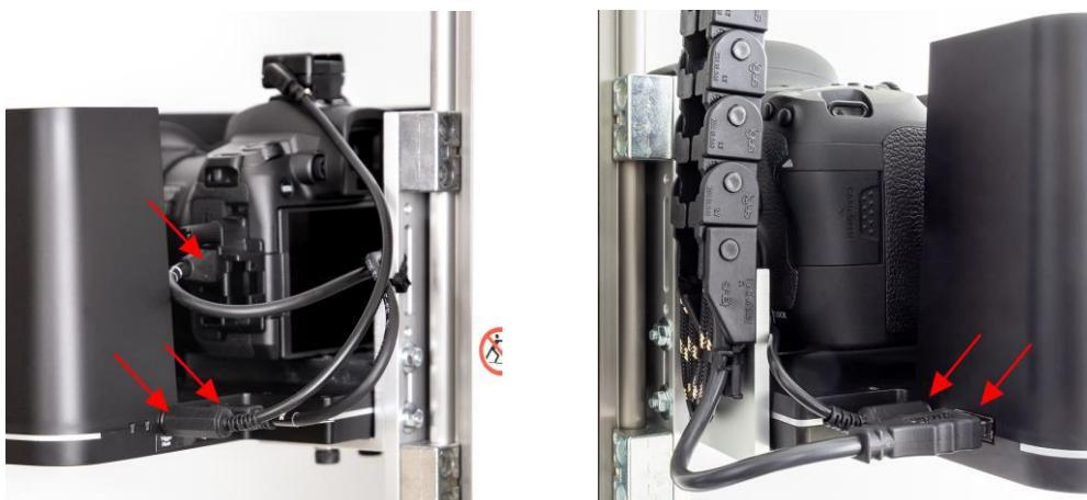
Fig. 19: Cable connections of PolFlash XE and camera to ATBM Tower (viewed from the left and right)
