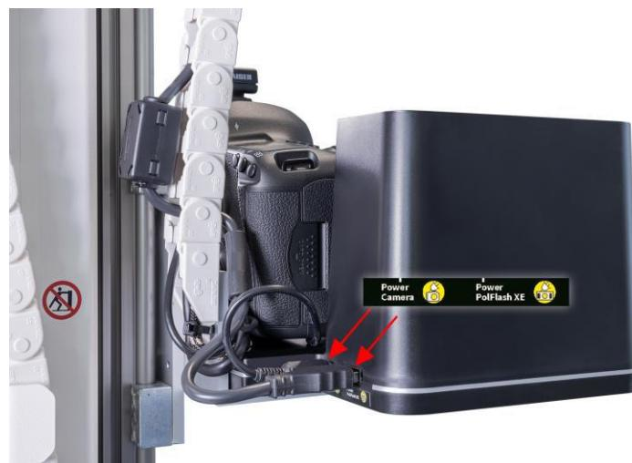
Fig. 16: Cable connections of PolFlash XE DX2 and camera to ATBM Tower (viewed from the right)
