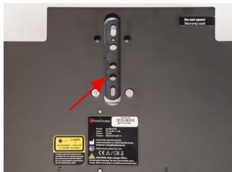
5. Screw on the camera from below through the corresponding screw hole of the positioning aid. Use the previously connected assembly material.
