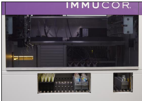
Hood in the down protective position
