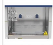
Work Zone Work zone, made of 304 stainless steel, is surrounded by negative pressure.
