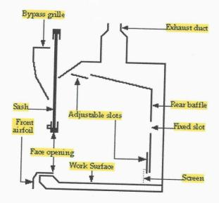
**Conventional/Constant Air Volume** - This is the most commonly used fume hood in our laboratories. The amount of exhausted air remains constant when the sash is in a full-open position. As the sash is lowered, the face velocity increases. **Floor-Mounted** - This type of hood is used when a large amount of working space
