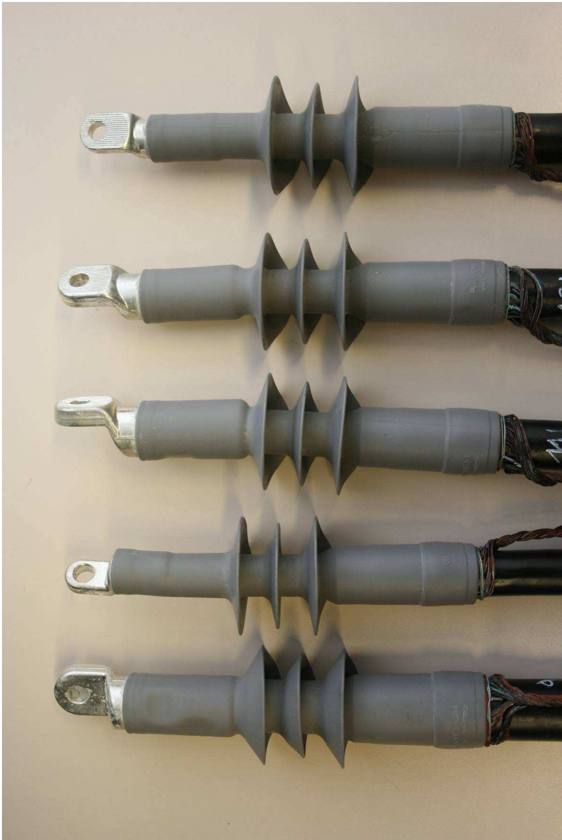
Picture 4: Terminations after humidity test
