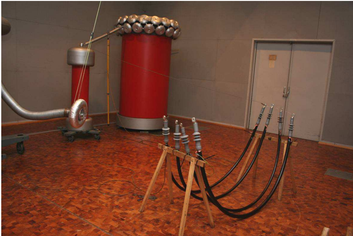
Picture 1: AC voltage withstand
