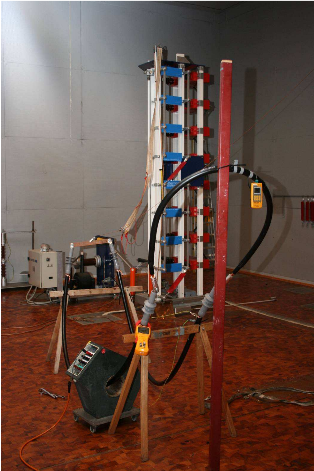
Picture 3: Impulse voltage at elevated temperature
