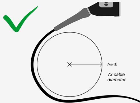
The cable must not be kinked or bent between the protective rubber sleeve and the camera head housing:
