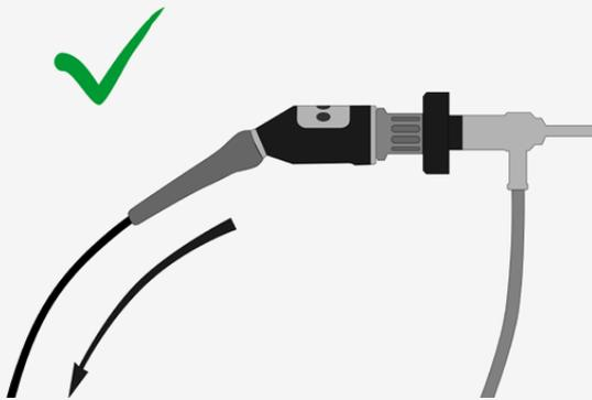
The protective rubber sleeve must not be removed:
