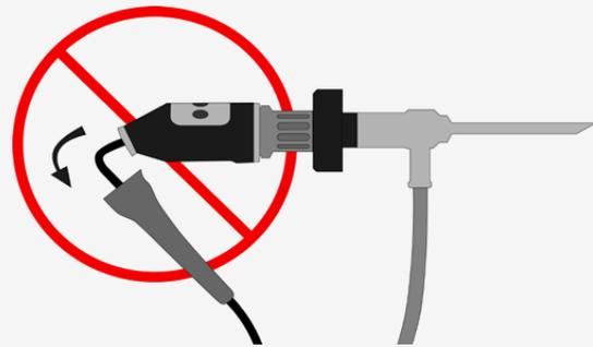
The cable and the protective rubber sleeve must not be kinked or bent sharply:
