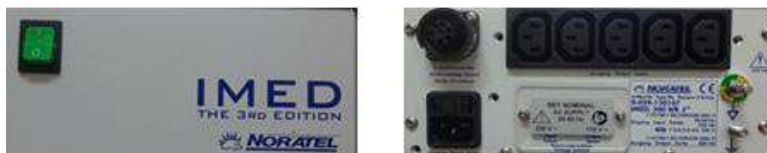
Figure 3-5. MED 300 WR (medical grade isolation transformer)
