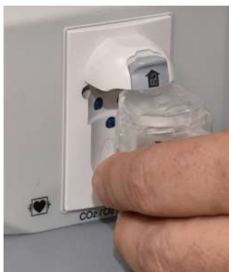
Fig. 6.1 Water trap installing
