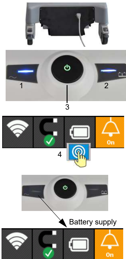
Fig. 3.2 Status LED supply
