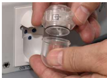
Fig. 6.2 Water trap replacement and emptying
