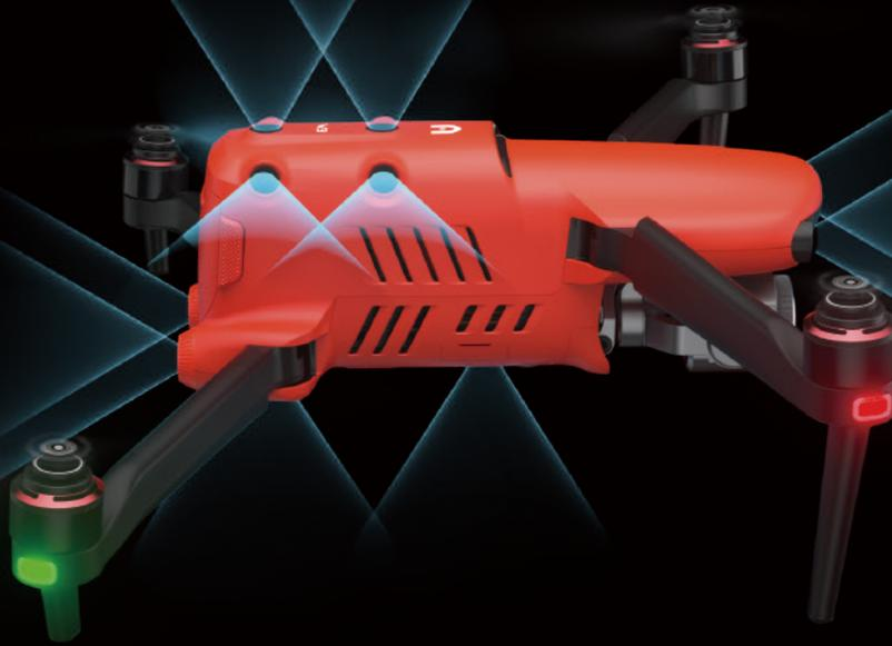
\*Please refer to the manual for details on obstacle avoidance and its limitations, which may or may not work in limited lighting environments, under direct strong sunlight, or across thin tree branches or wires.
