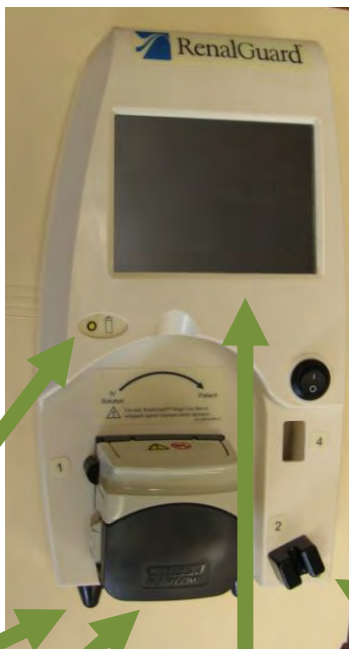
Figure 15 Front Enclosure Battery LED Feet Pump Head Display/Touchscreen Air Detect On/Off Switch
