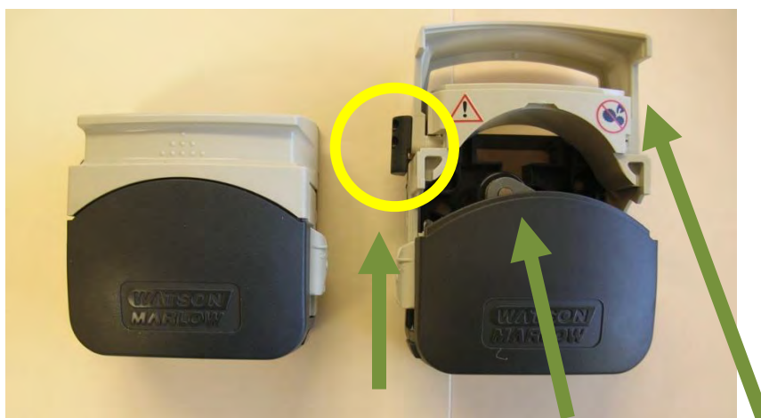
Figure 22 Pump Head Assembly Magnetic Holder Pump Rollers Pump head Door
