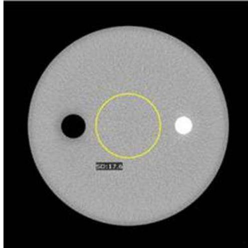
Fig 12-4 Noise Measurement of Body Phantom Using Body STD-QA Protocol
