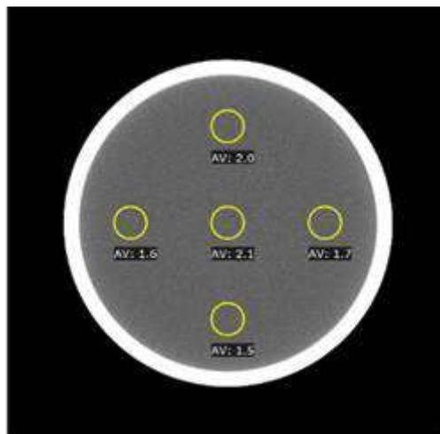
Fig 12-7 CT Value Uniformity Measurement of Water Phantom Using Head STD-QA Protocol
