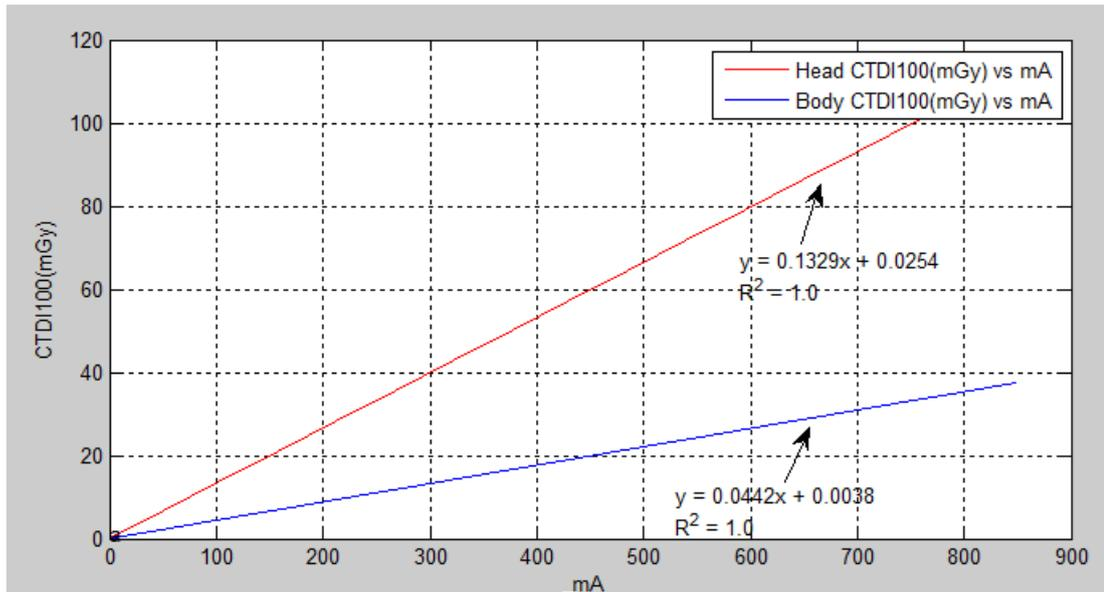
Fig 14-3 Linearity of X-ray Output Dose for Large Wedge
