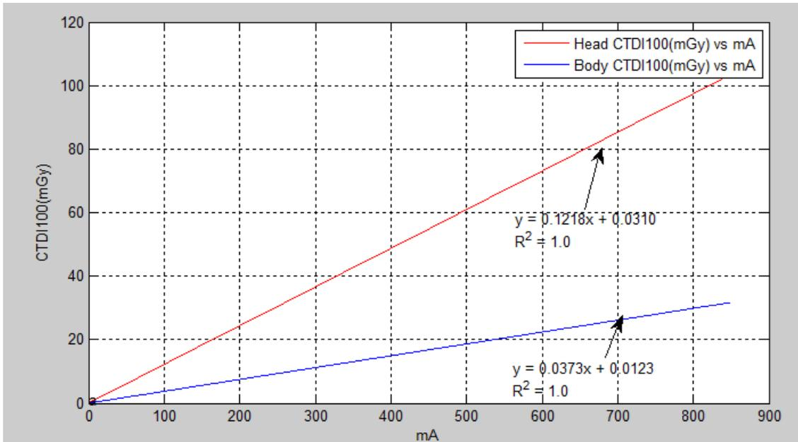
Fig 14-4 Linearity of X-ray Output Dose for Medium Wedge
