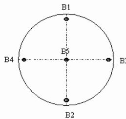
Fig 14-1 Position Schematic Diagram of Measuring the CTDI Dose
