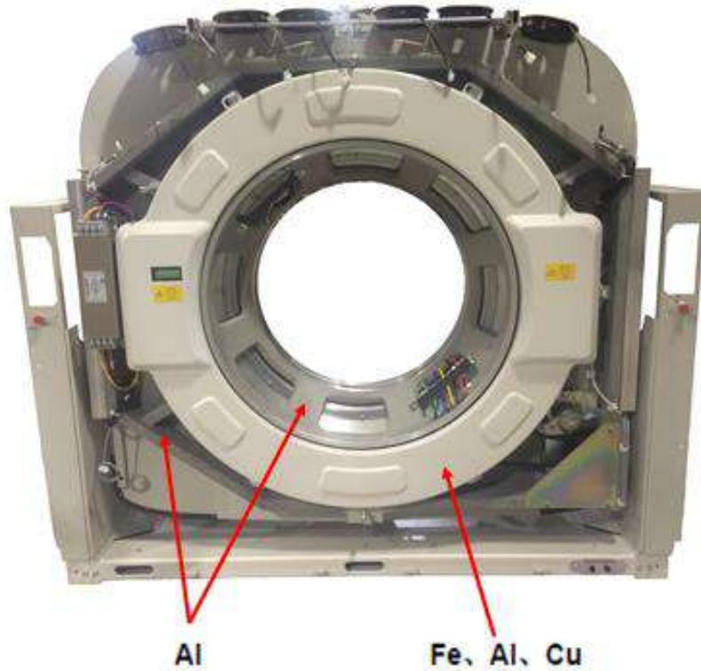
Fig 15-4 Gantry Rear View (Without Cover)
