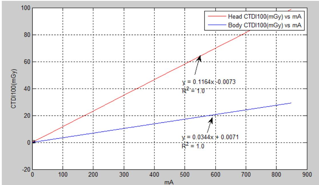
Fig 14-5 Linearity of X-ray Output Dose for Small Wedge
