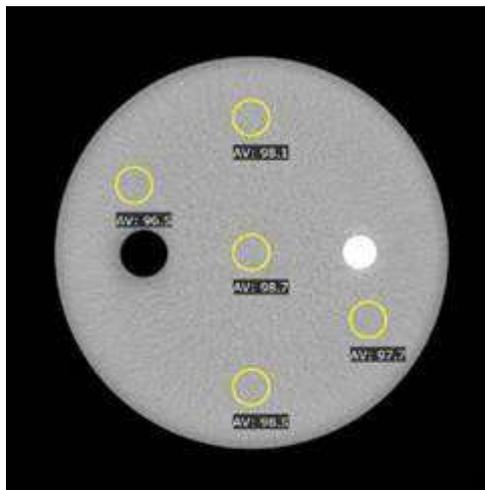
Fig 12-8 CT Value Uniformity Measurement of Body Phantom Using Body STD-QA Protocol
