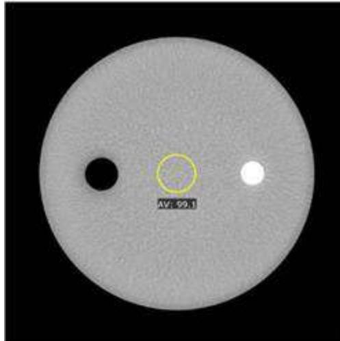
Fig 12-6 CT Value Measurement of Body Phantom Using Body STD-QA Protocol
