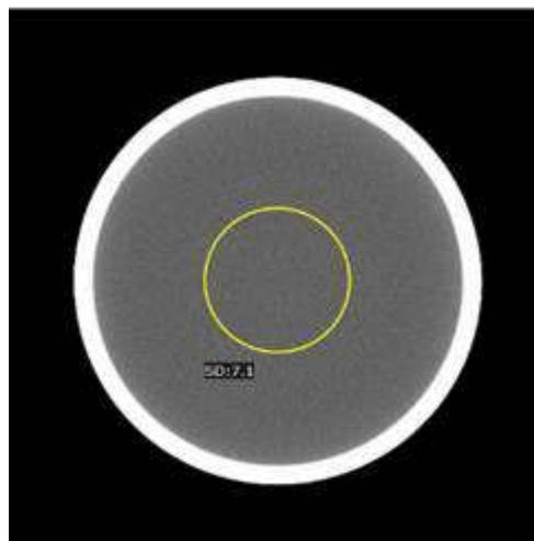
Fig 12-3 Noise Measurement of Water Phantom Using Head STD-QA Protocol
