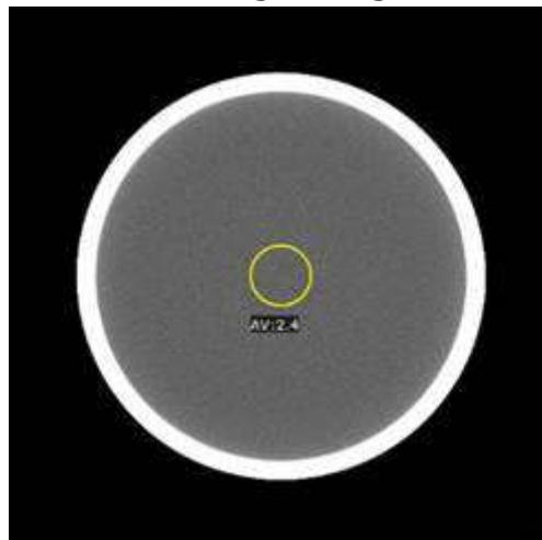
Fig 12-5 CT Value Measurement of Water Phantom Using Head STD-QA Protocol
