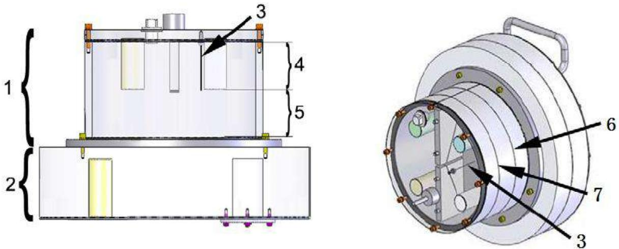
Fig 12-1 QA Phantom Composition
