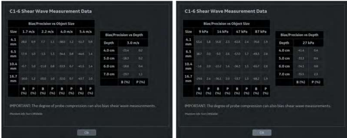
Figure 13-50. C1-6-D/C1-6VN-D Measurement Bias Information (Velocity on the left and Stiffness on the right)
