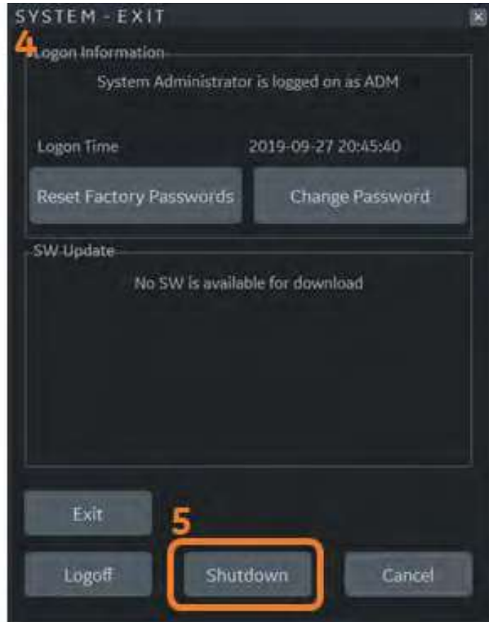
Figure 13-274. Shutdown to Begin Installation
