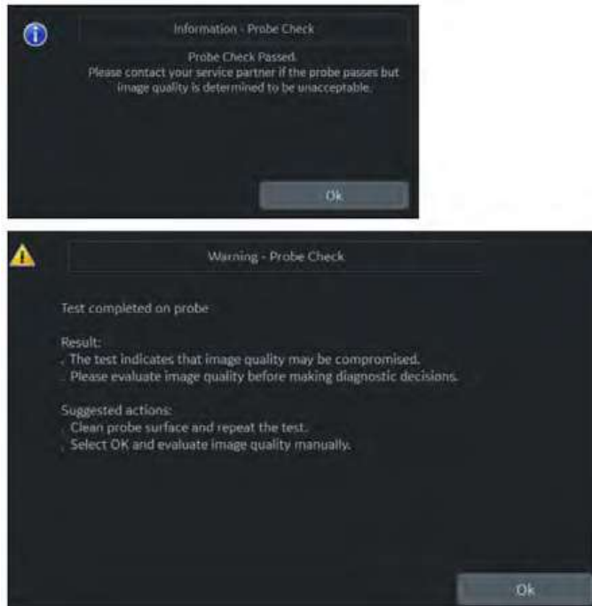
Figure 11-19. Probe Check Pass or Fail Pop-ups
