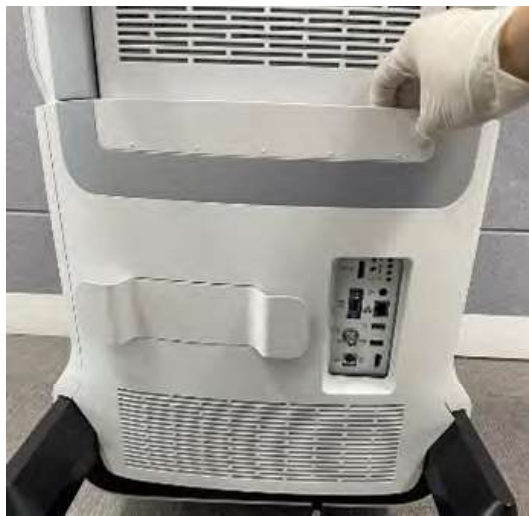
Figure 12-9. Remove the rear cover
