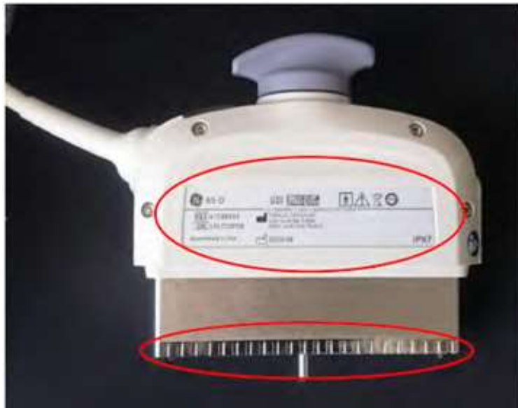
Figure 11-8. Connector/console interface surface and label
