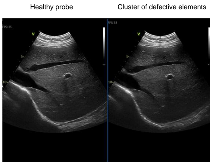
Figure 13-25. Example of image degradation for a curved probe
