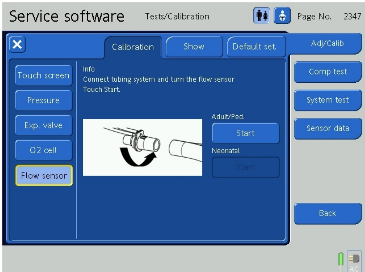
Figure 8-43. Adult/Ped. flow sensor calibration (Page No. 2347)
