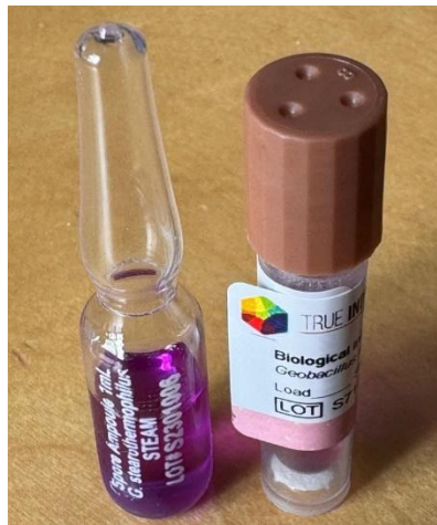
Figure 1. Commercial vials containing spores in liquid form (left) or enclosed in a carrier (right). At the bottom of the vial on the right, the paper disc containing the spores is clearly visible.
