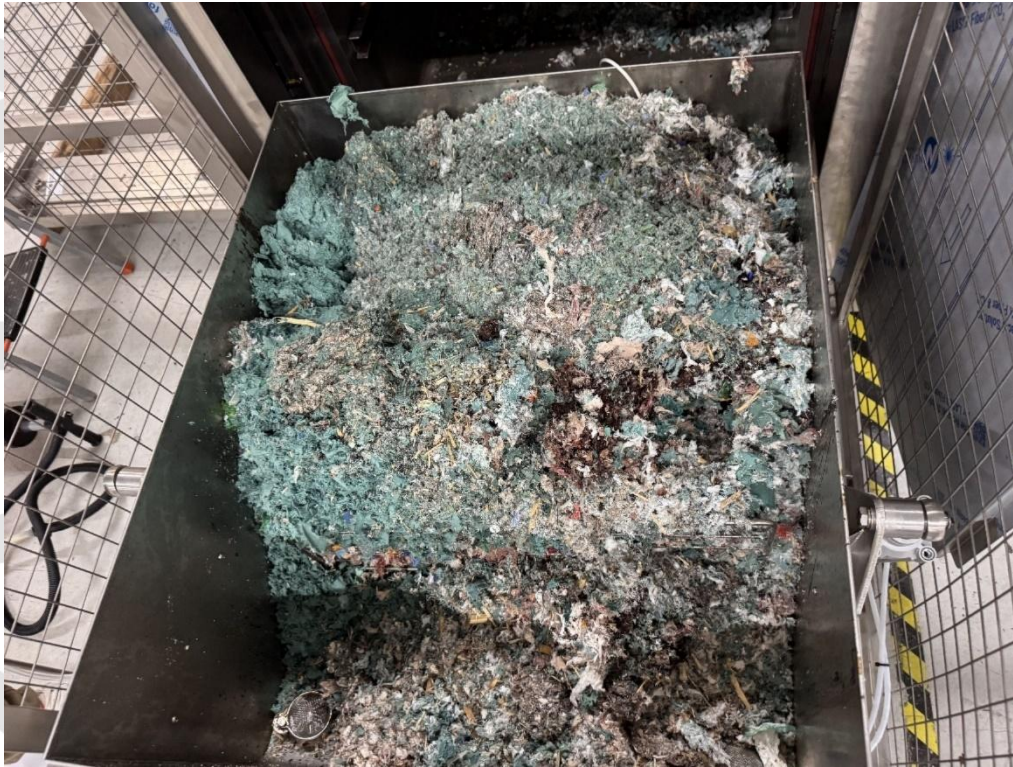
Figure 4. Shredded and sterilized waste at the end of a full load cycle.
