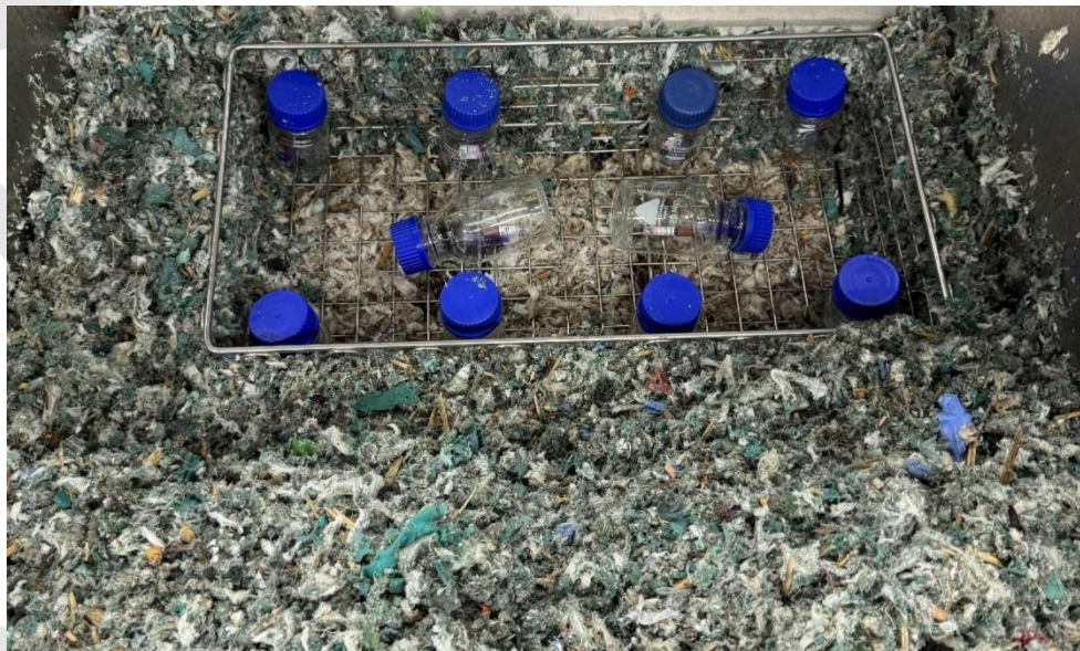
Figure 6. Bottles containing spore vials before being covered with shredded waste.
