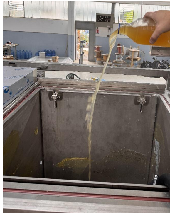
Figure 5. Addition of the lactic bacteria solution through the shredding chamber.
