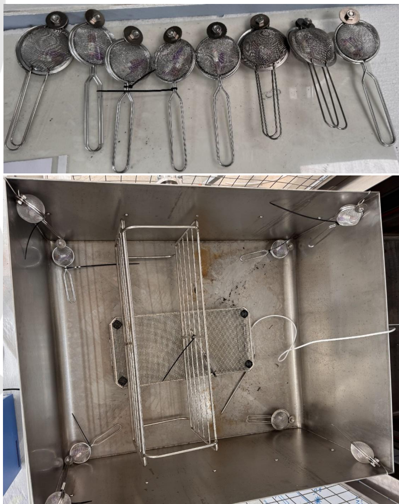
Figure 3. Sieves containing the vials (above) and their positioning inside the container for collecting shredded waste.
