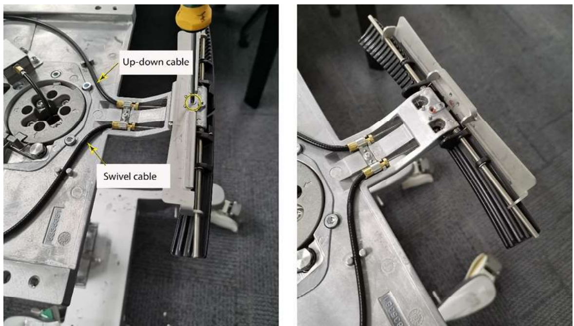
Figure 8-128 Protective Metal Plate Rotated 90 Degrees
