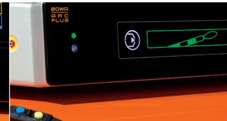
The green display signals pre-flushing of the connected instruments with argon
