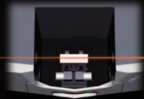
Flame measurement: Burner head intersects the light axis (red line).
