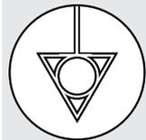
Connect a potential equalization conductor as per IEC 60601-1.
